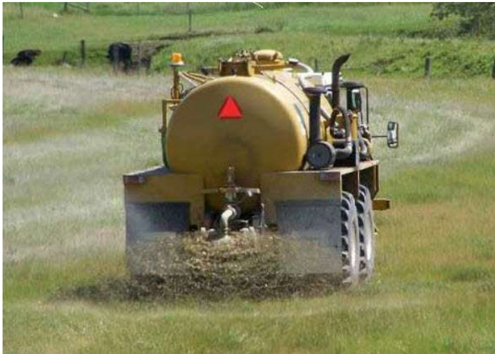
Figure 10-1. Surface Application of Septage Waste
