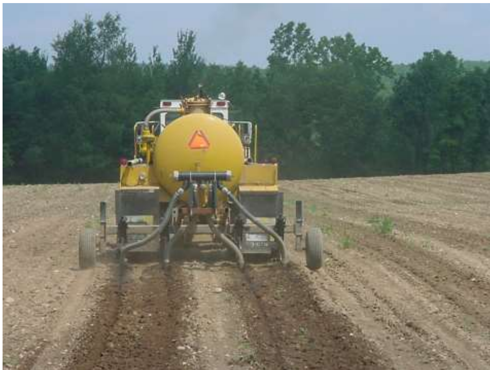
Figure 10-2. Subsurface Injection of Septage Waste
