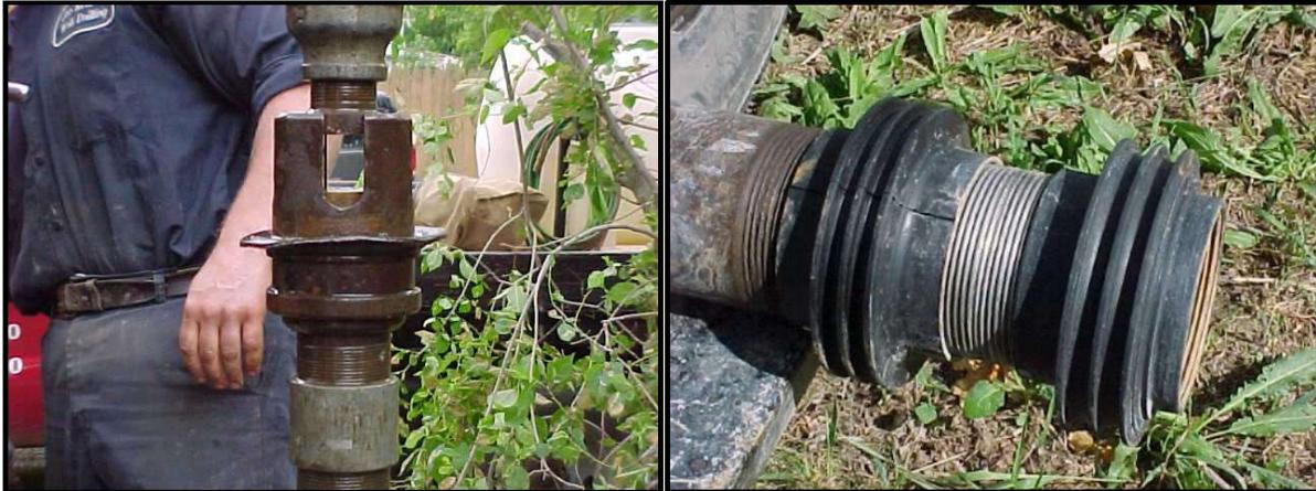
The force exerted on the formation depends on the length of the stroke and the vertical velocity of the surge block.
