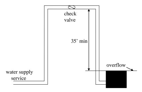
Figure 4-14 Barometric Loop
