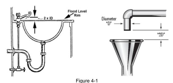
Air gaps have proven to be an effective method of protecting against backsiphonage in common household installations such as sinks, bathtubs, washers, and water softeners as well as hazardous industrial applications. Air gaps are not testable but need to be inspected from time to time to make certain that someone has not altered the plumbing.
