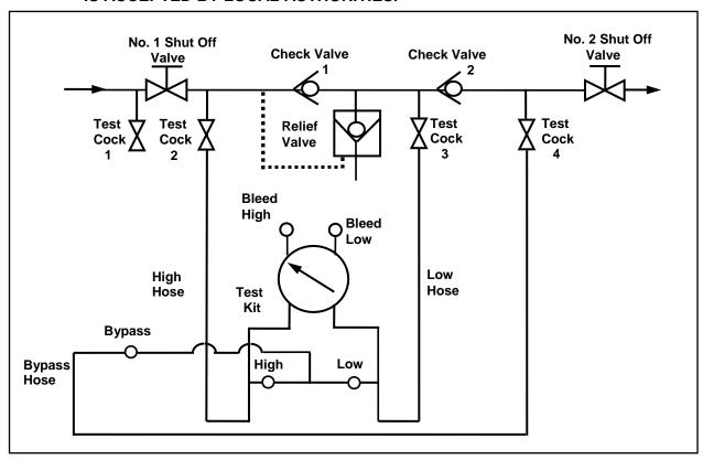
**TEST SET UP:**
