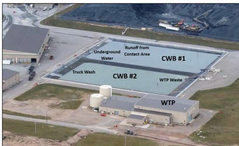
Figure 5 – Layout of the CWB's
