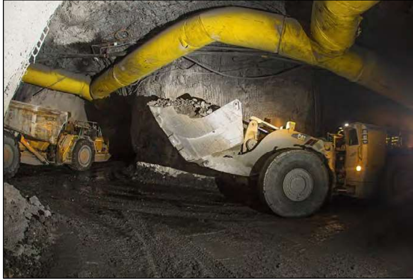
Figure 2 – Haul Truck Loading Material Underground
