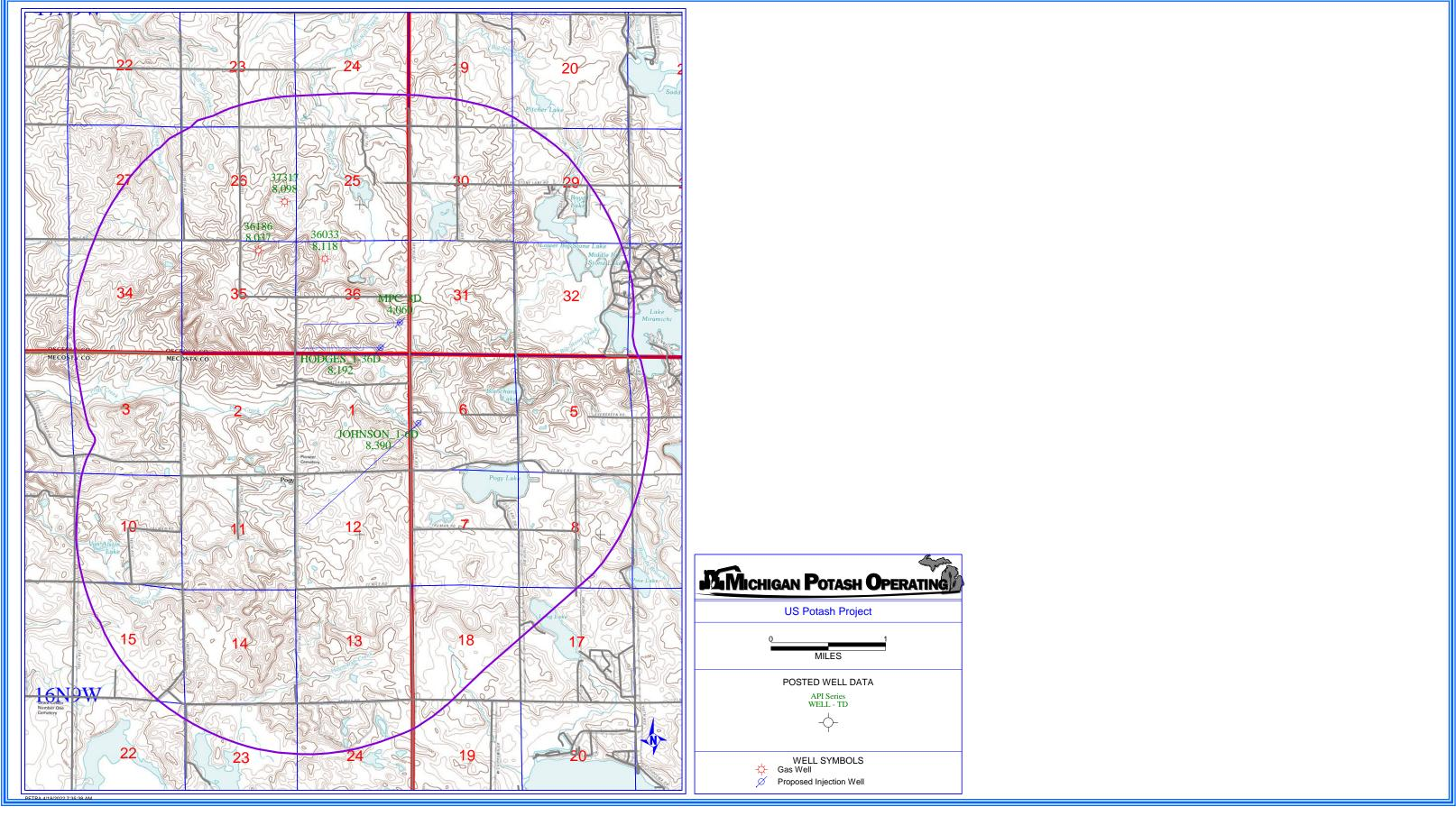
Figure A4 . Map showing all producing wells in relation to the proposed injection wells. Public Land Survey System is included. A blue box measures one section, or one square mile.
