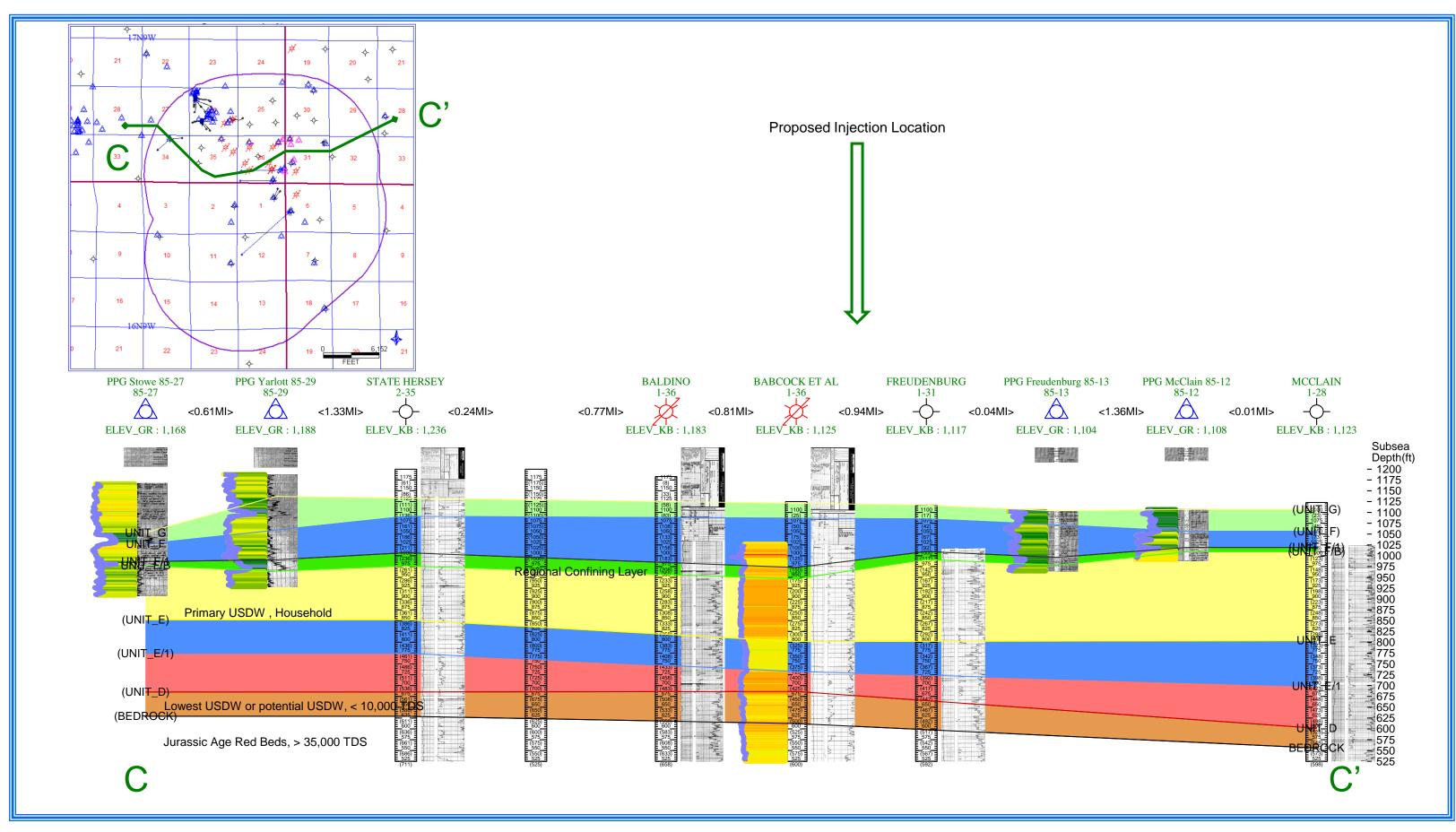
Figure B10. A cross section extending across the entire AOR, spanning an approximate 5.5 mile length from West to East, crossing the reference wells utilized in Figure D5. The cross section path can be referenced by the small map in the upper left hand corner.
