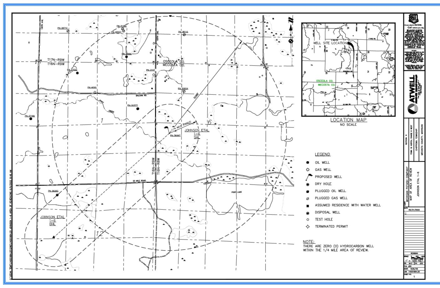
Figure A8. Plat showing third party survey, with a ¼ mile area around the well path. Also showing a 1 mile radius from the wellhead locaiton. There are no oil and gas operators within the ¼ mile length of the subject well, or within the one mile boundary beyond the facility property boundary. The plat also illustrates the project injection well(s), well pad(s).
