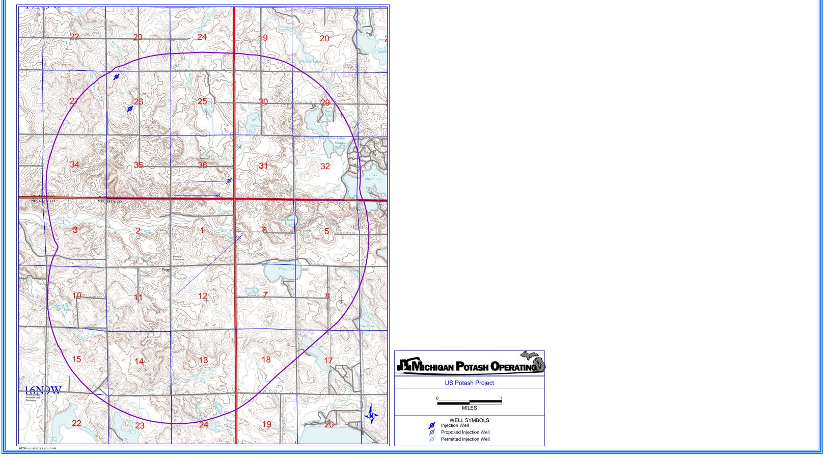
Figure A5. Map showing Existing Class I NON-HAZARDOUS Injection Wells, the Thomas 1-26 (NW4NW4 Section 26) and the Woodward 1-26 (NE4SW4 Section 26). Also shown are permitted injection wells the MPC 1D, MPC 2D, and MPC 3D. The Proposed 8D shares a pad location with the MPC 3D.
