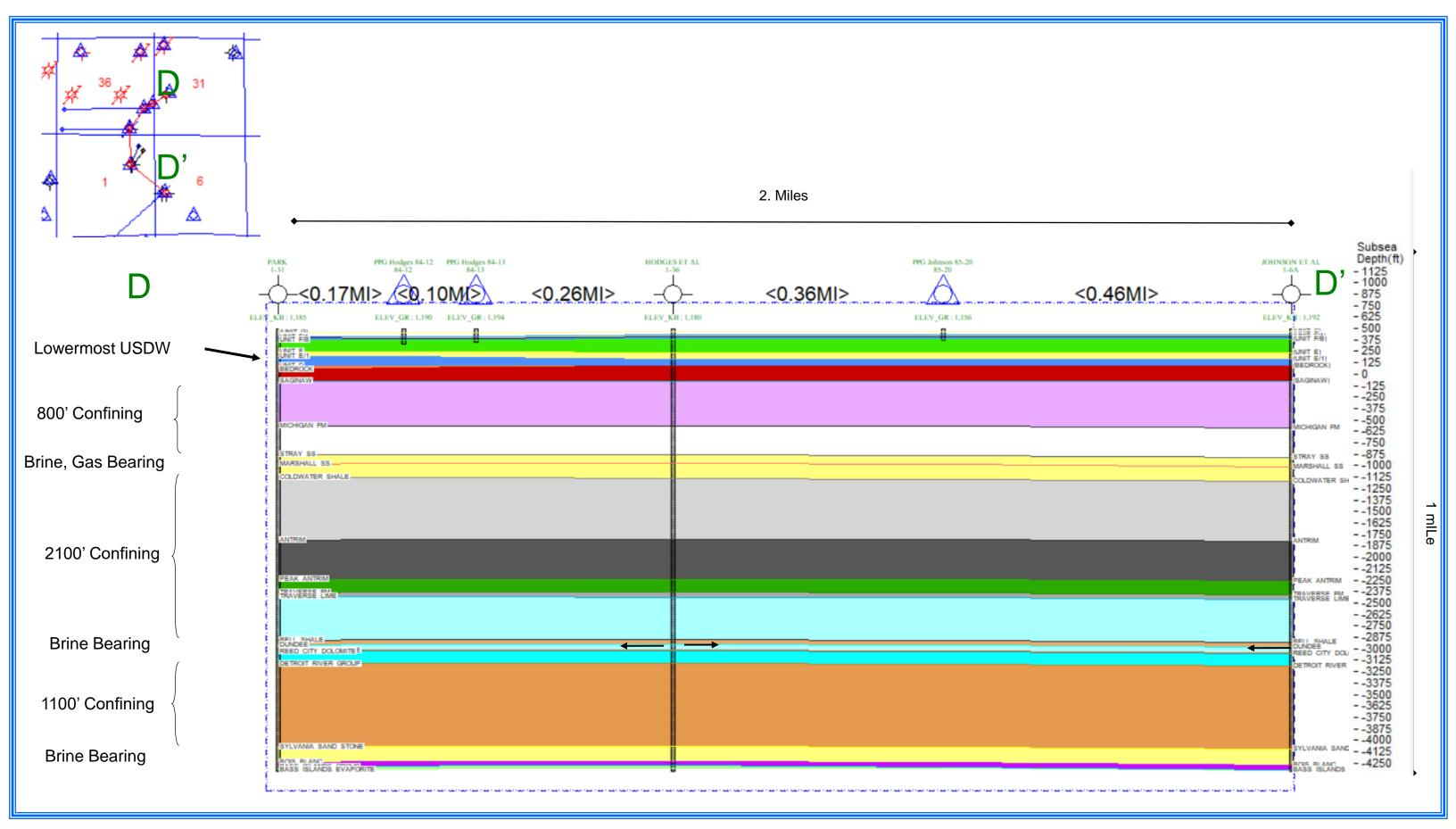
Figure B1 shows the USDWs in relation to the proposed injection zones in the immediate proximity of the PROPOSED WELLBORES. The larger cross section is intentionally shown on a 1:1 ratio, with no vertical exaggeration to illustrate the amount of inte-rlayered and non-permeable intervals between any potential injection zone and any potential USDW.
