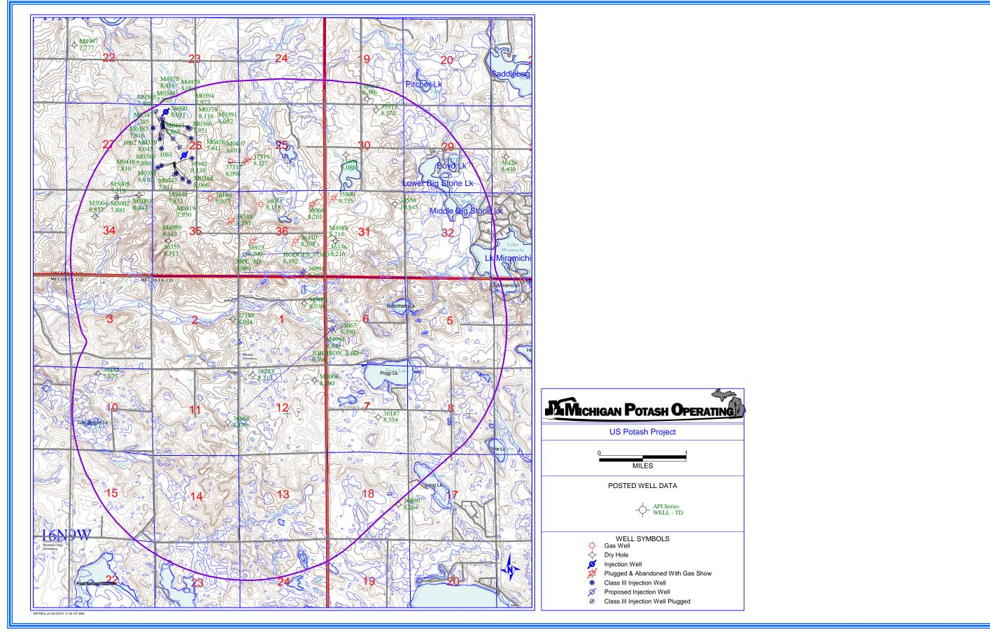
Figure A9. Map showing all well types, active and inactive, within the Area of Review. Shown in blue highlight are surface water bodies. Roads are also shown (black). PLSS is also shown (Blue). Well API series, and Total Depth are listed in GREEN. Mineral Wells are preceded with an M.
