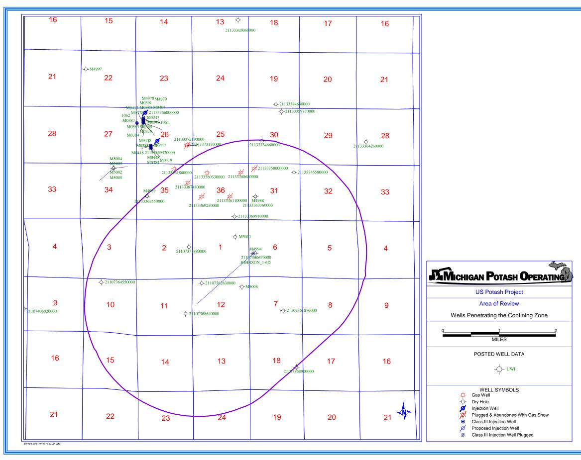
Figure A2 is a map illustrating a 2 mile radius along the lateral trajectory of the Johnson 1-6D, also showing the PLSS system and all deep wells that penetrate the confining horizon.
