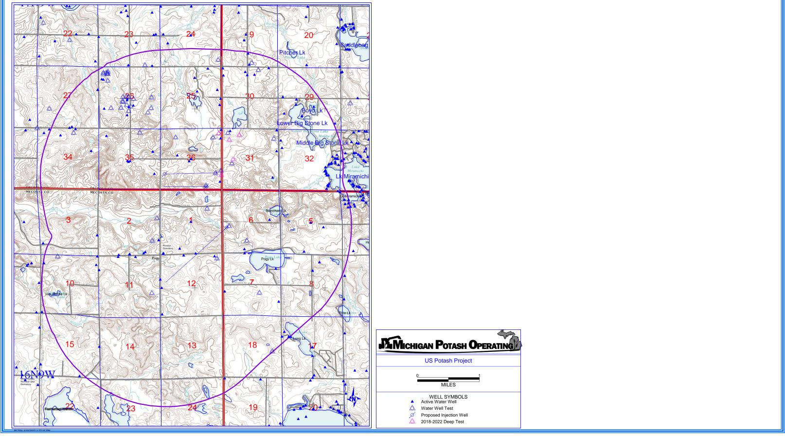
Figure B4. Map showing hydro-geological investigation wells, and water wells, and recent 2018-2022 hydrological investigation wells (some, not all) drilled for the sole puporse of understanding, in order to protect, the groundwater and USDW within the AOR.
