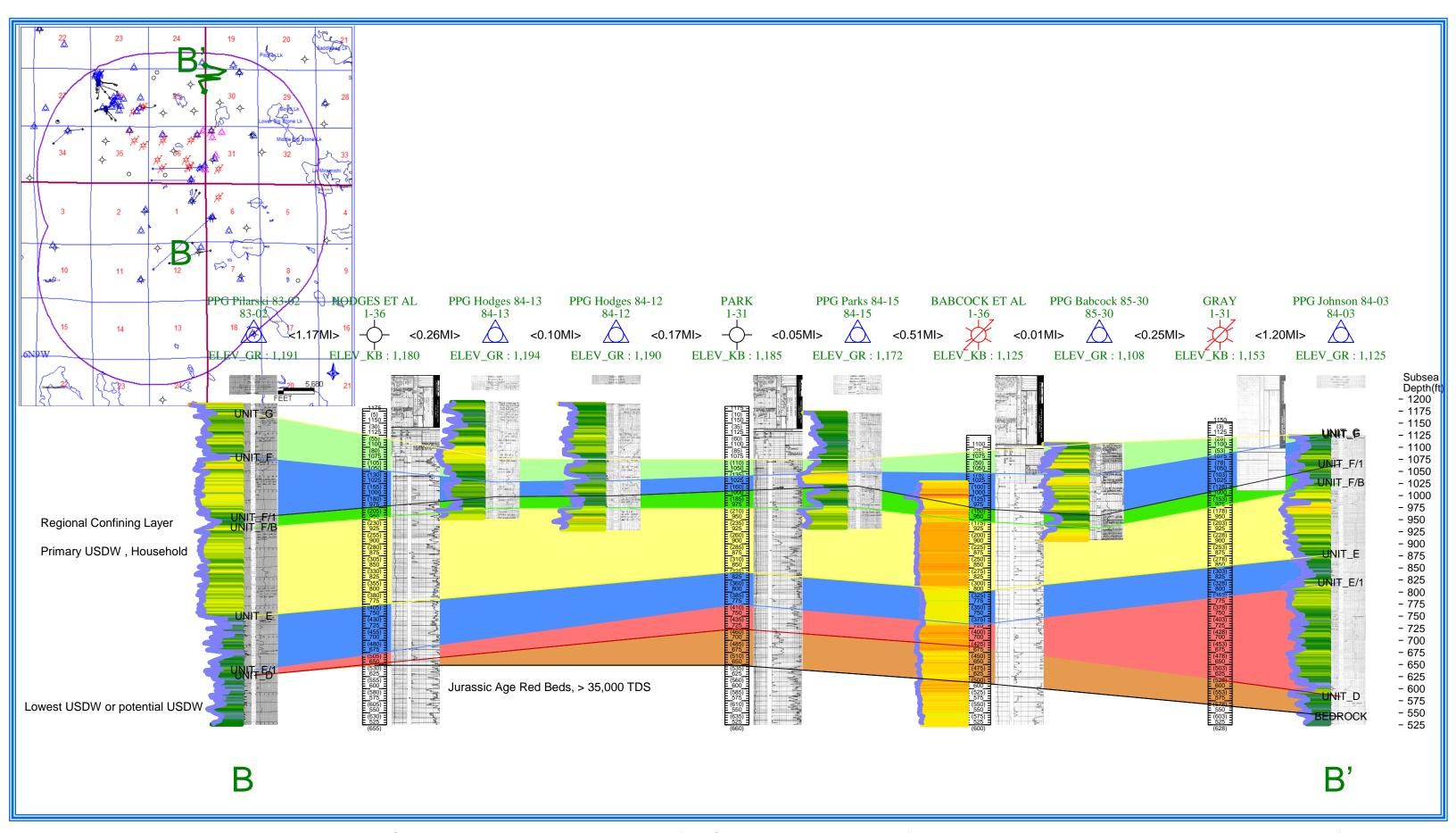
Figure B9 is a cross section extending across the entire AOR, spanning an approximate 3.5 mile length from South to North, crossing the reference wells utilized in Figure D5. The cross section path can be referenced by the small map in the upper left hand corner.
