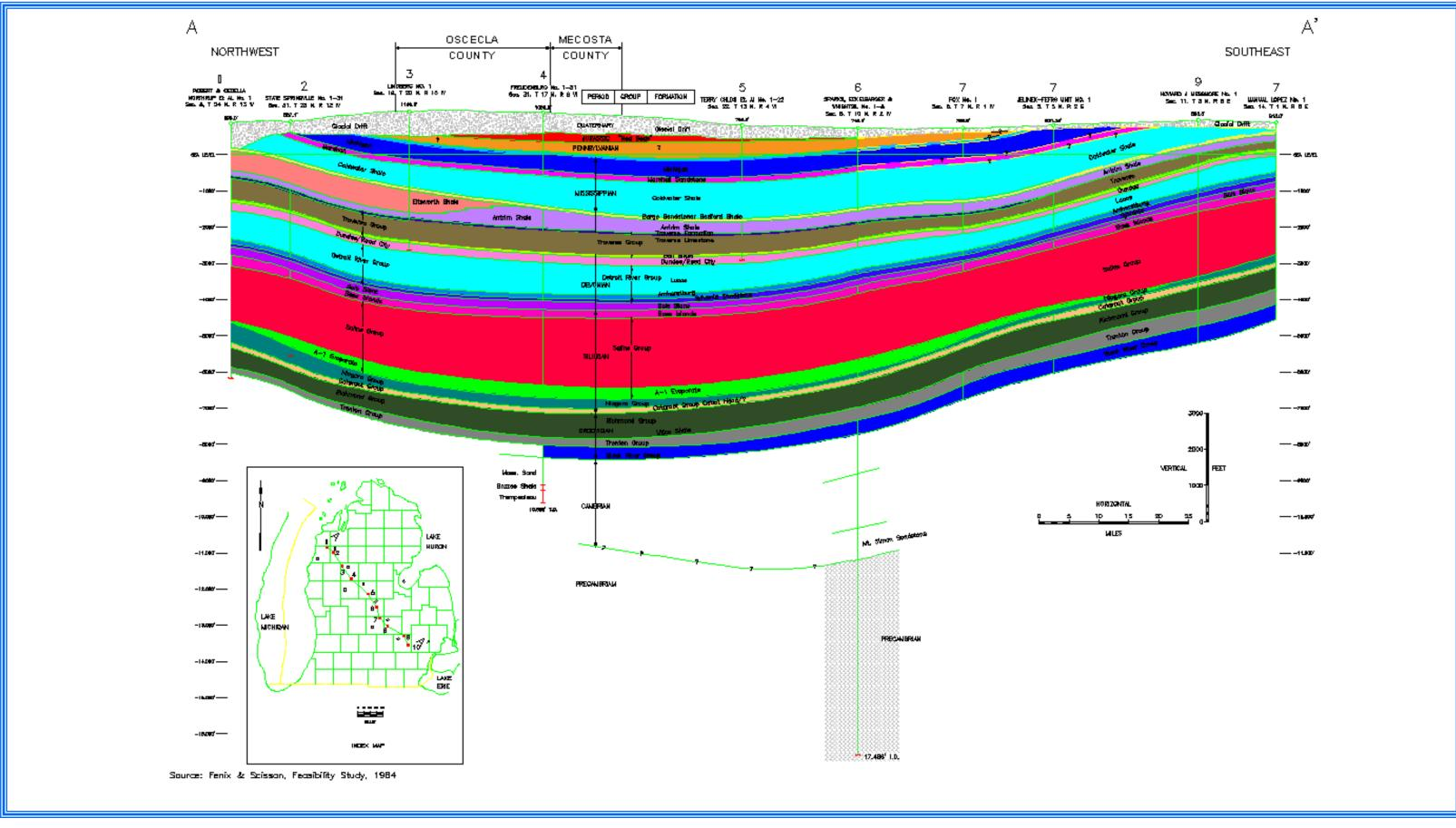
Figure C3. A detailed northwest-southeast regional cross-section through the estate of Michigan, drawn through the AOR, utilizing the deepest well in the AOR (Fruedenburg 1-31 - 10,858 feet), which is in the same section as the proposed injection location (Section 31, Evart Township, Osceola County, Michigan).
