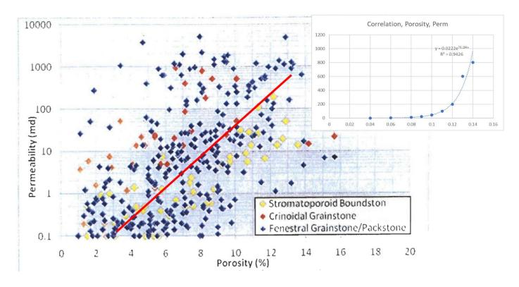
A site specific porosity crossplot of the Netron Density and Bulk Density over the Park 1-12, which is the target toe locaiton of the Johnson 1-6D directional plan, demonstrates fully dolotimized Dundee in the Reed City Member, and high effective porosity. This would be indicative and corroborative of the high measured permeability via DST testing in the offset Ward 1-11 (>350 md), and the injection step rate testing in the Woodward and Thomas (>900 md).
