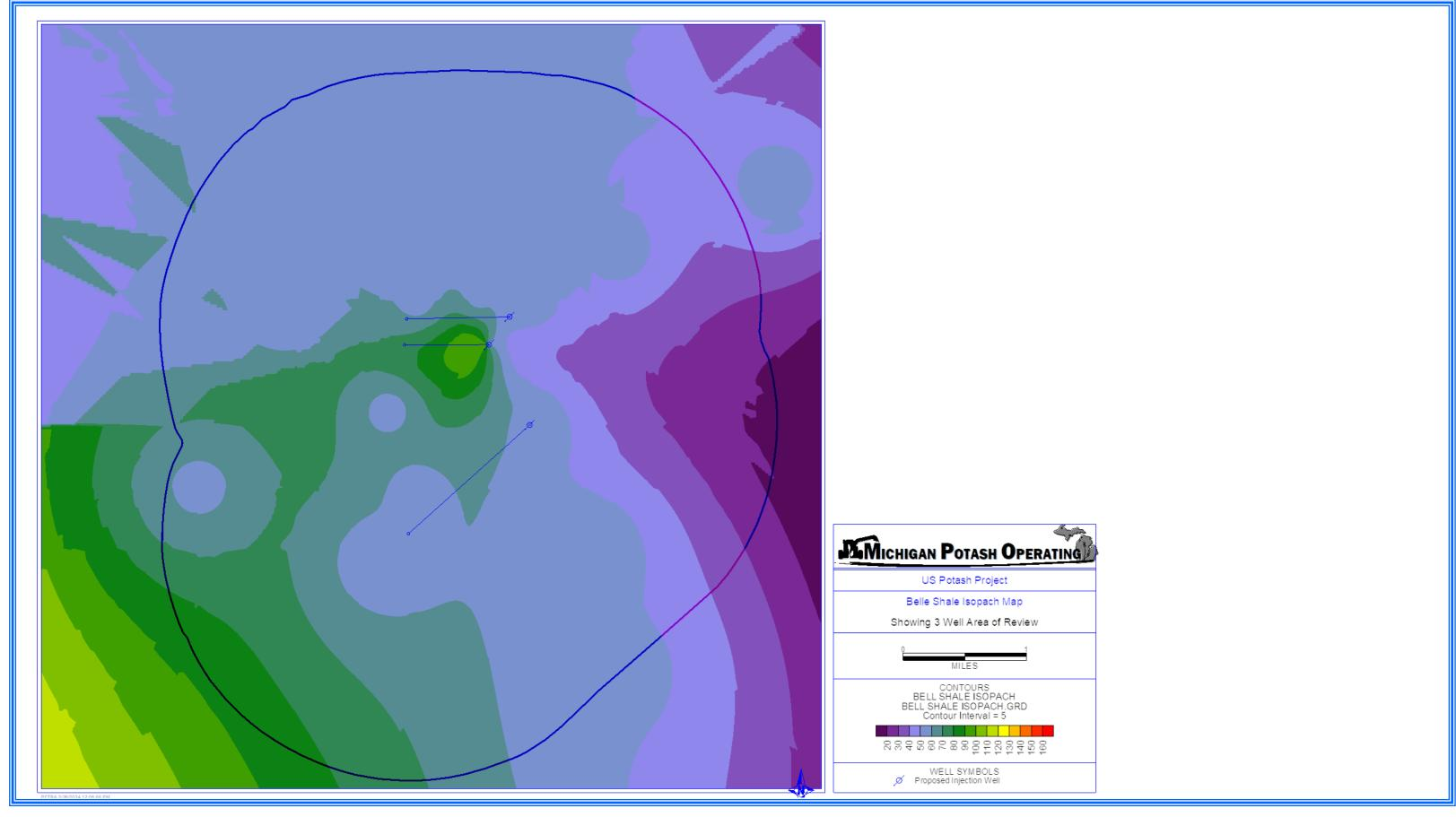
Figure C13. An isopach map of the Belle Shale.
