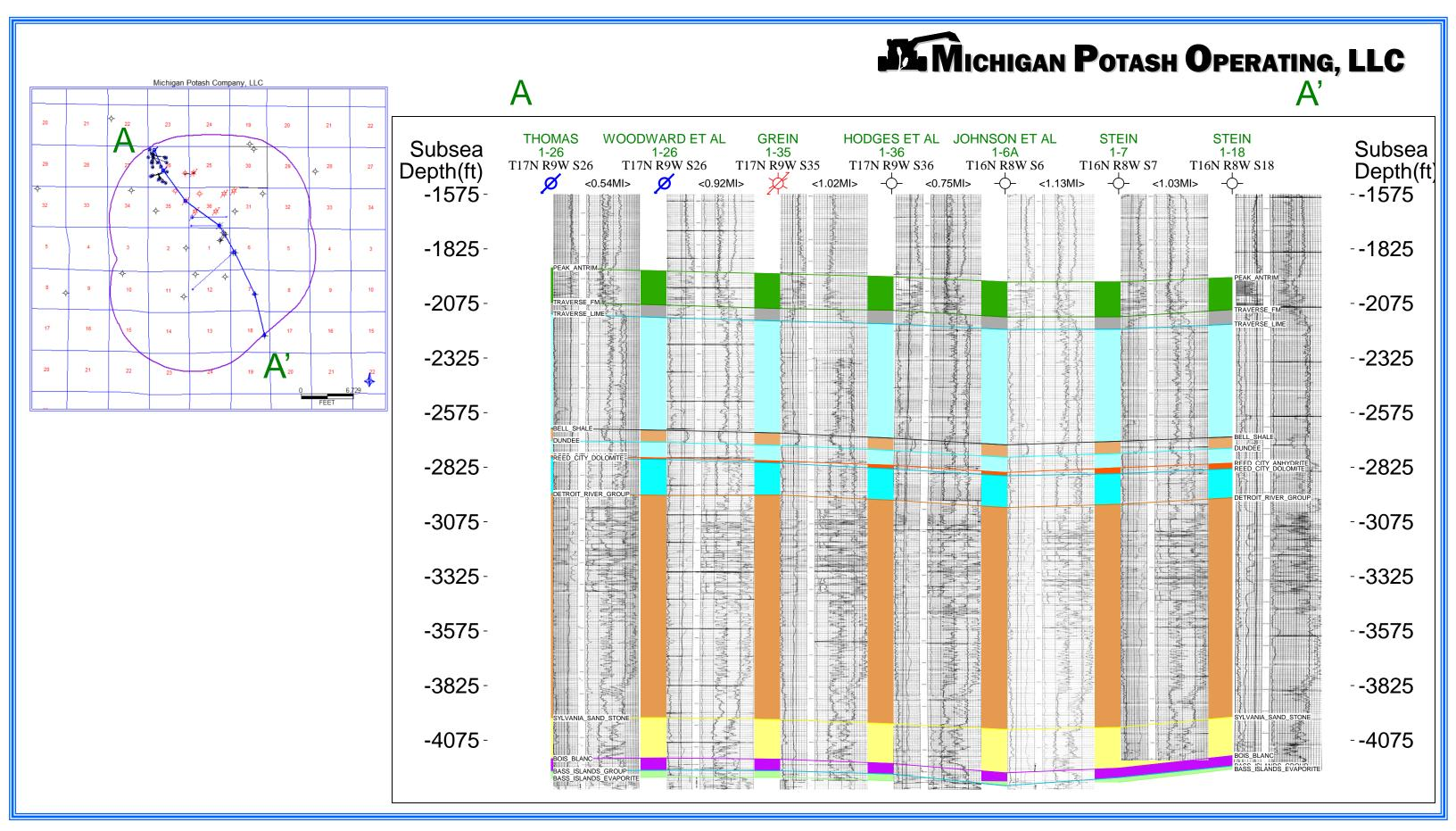
Figure C5 is a cross section through the AOR, showing the geological units of interest and their immediate confining layers from North West (A) o South East (A').
