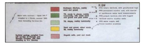
Figure B3. A surfical geological soil map compiled from soil surveys from over 308 hydrological test holes and approximately 60 piezometers cataloging over 33,833 feet of groundwater and soil data compiled by W.A. Menley over the AOR. Contours showing the observed water table of the Upper Unit F are shown on top of the soil catalogue. Each of the proposed wells are shown..
