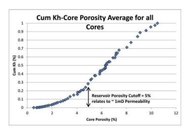
Cumulative permeability-feet percent (Cum Kh) versus core porosity average for all 26 wells with whole-core analysis reports. Average core porosity 0%–12% is located on *x* axis, and cumulative permeability-feet (decimal percent) 0–1 is on *y* axis. The inflection point occurs at 5% porosity and was used as a reservoir cutoff. This reservoir cutoff value may define economically producible hydrocarbons from noneconomical hydrocarbons.
