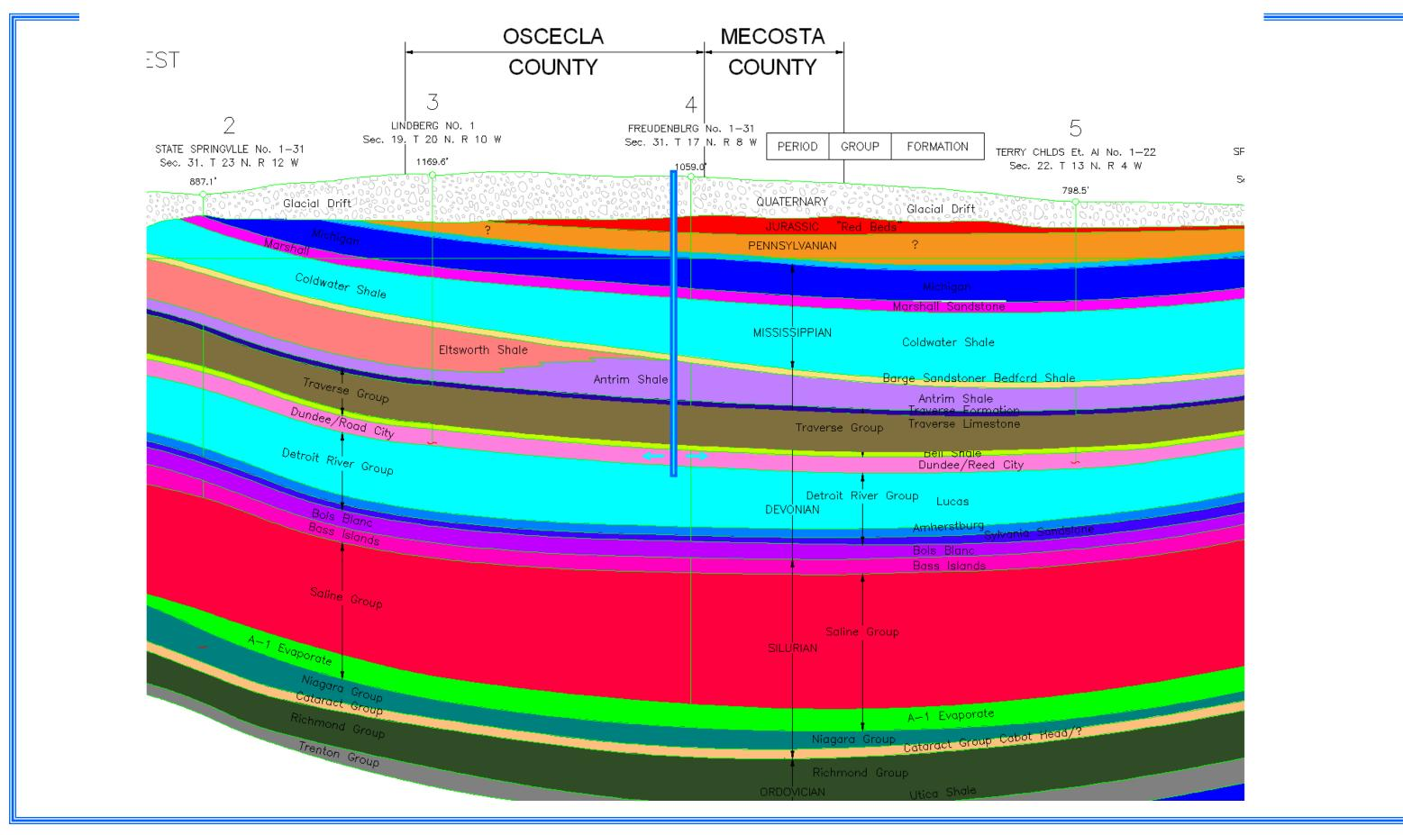
Figure C4 is a zoomed in portion of Figure B5, showing the proposed injection horizon in relation to its stratigraphic column.
