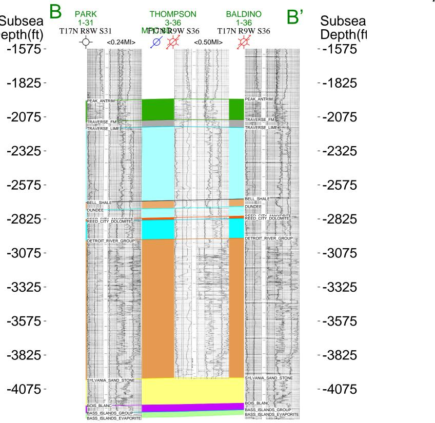
Figure C7 is a cross section tracing the MPC 8D and Hodges from East (B) to West (B')..
