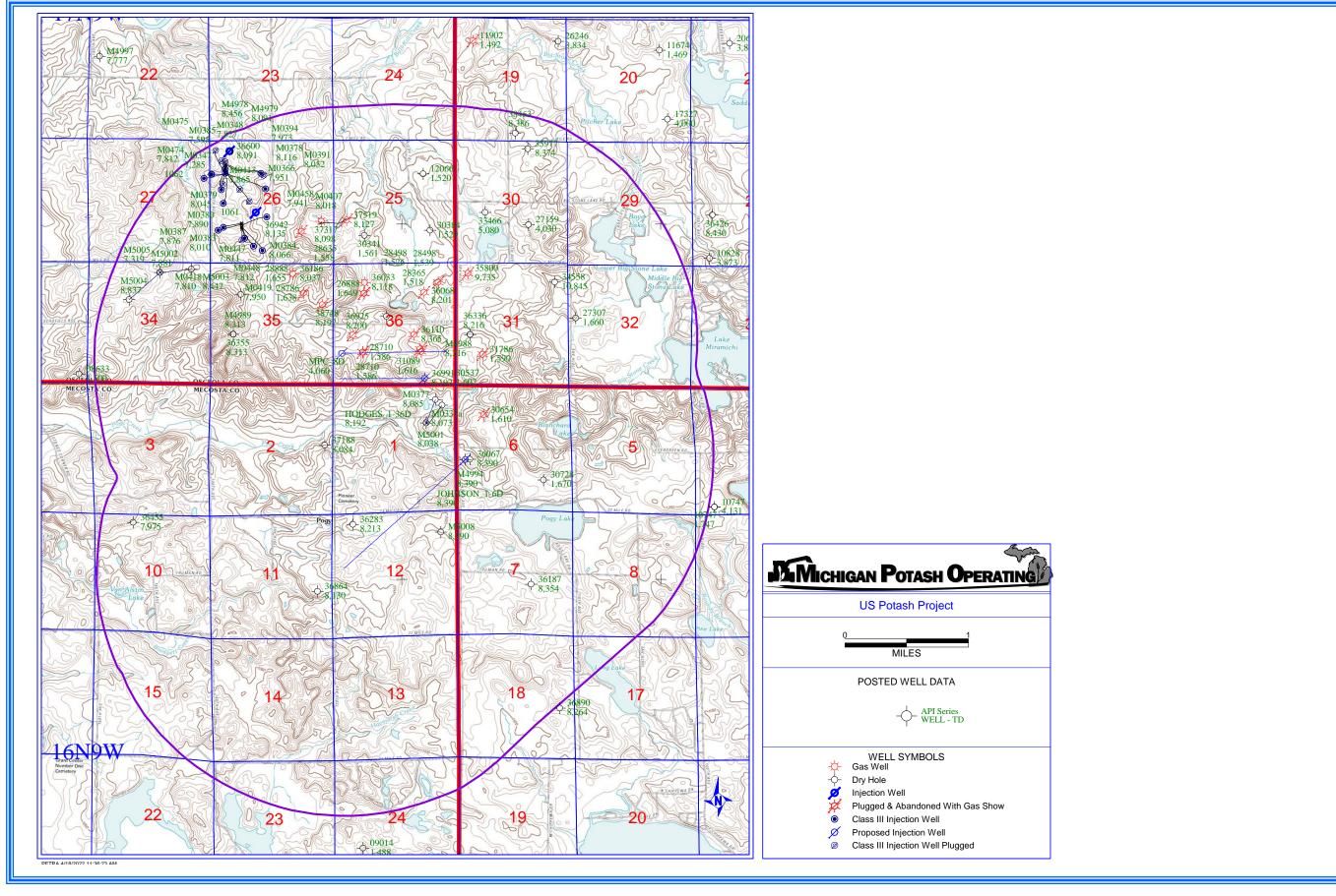
Figure A7. Map showing all plugged wells, shallow (that do not penetrate any confining horizon) or deep (that penetrate confining horizon) within the area of review. Total Depths are listed. There are several shallow Michigan Stray wells that do not penetrate the injection or confining horizon.
