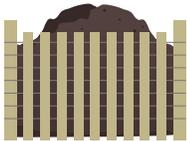
**Snow Fence Bin:** Buy a length of prefabricated snow fence and fasten 2x4s to each corner to form a square. For a 4' x 4' x 4' compost pile, purchase 16 feet of snow fencing.
