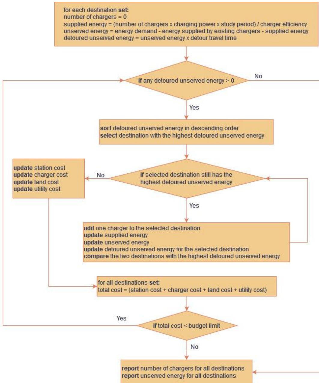
Figure 12. Flowchart of heuristic approach for Level-2 charger allocation
