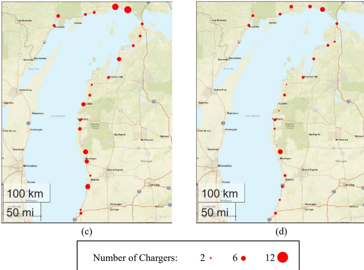
**Figure 18. Optimal charging infrastructure configuration under (a) No budget limitation (b) \$8 million budget (c) \$6 million budget (d) \$4 million budget**
