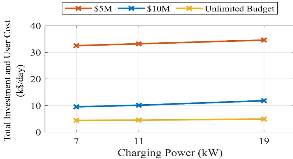
**Figure 15. Total investment and user cost per charging power for different budget limits**
