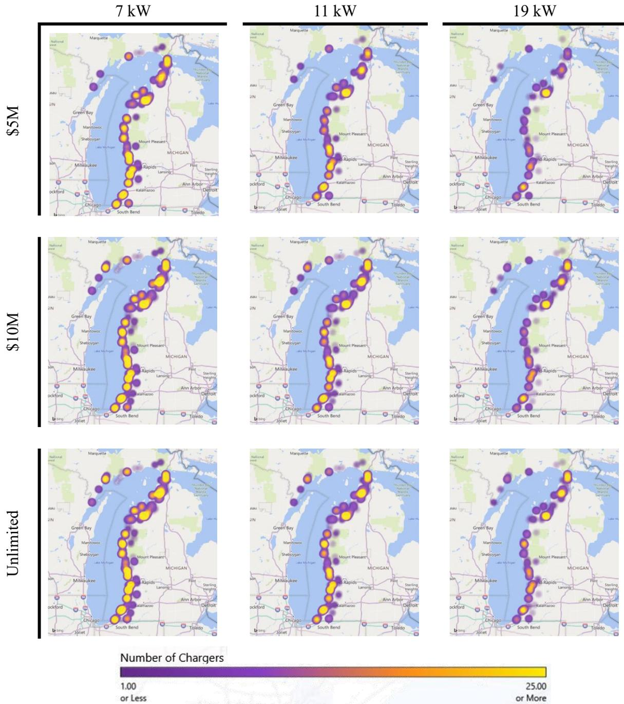
**Figure 17. Distribution of Level-2 chargers in LMC area for different budget limits and charging powers**
