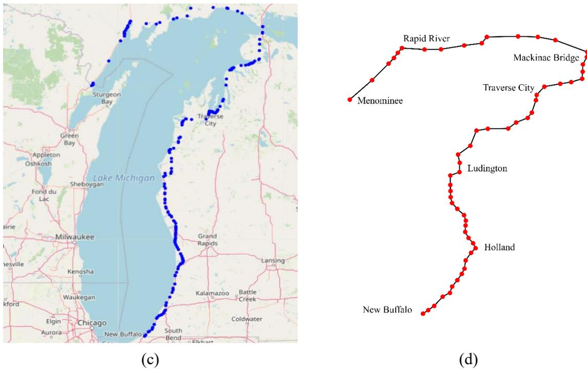
**Figure 5. Corridor Node Identification Process: (a) DCFC Candidate Locations (b) Distribution of Candidate Locations (c) Corridor Access Points for Candidate Locations (d) Final LMC Corridor Nodes**
