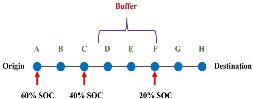
**Figure 14. An Illustrative Example Demonstrating the Purpose of the Buffer Range**
