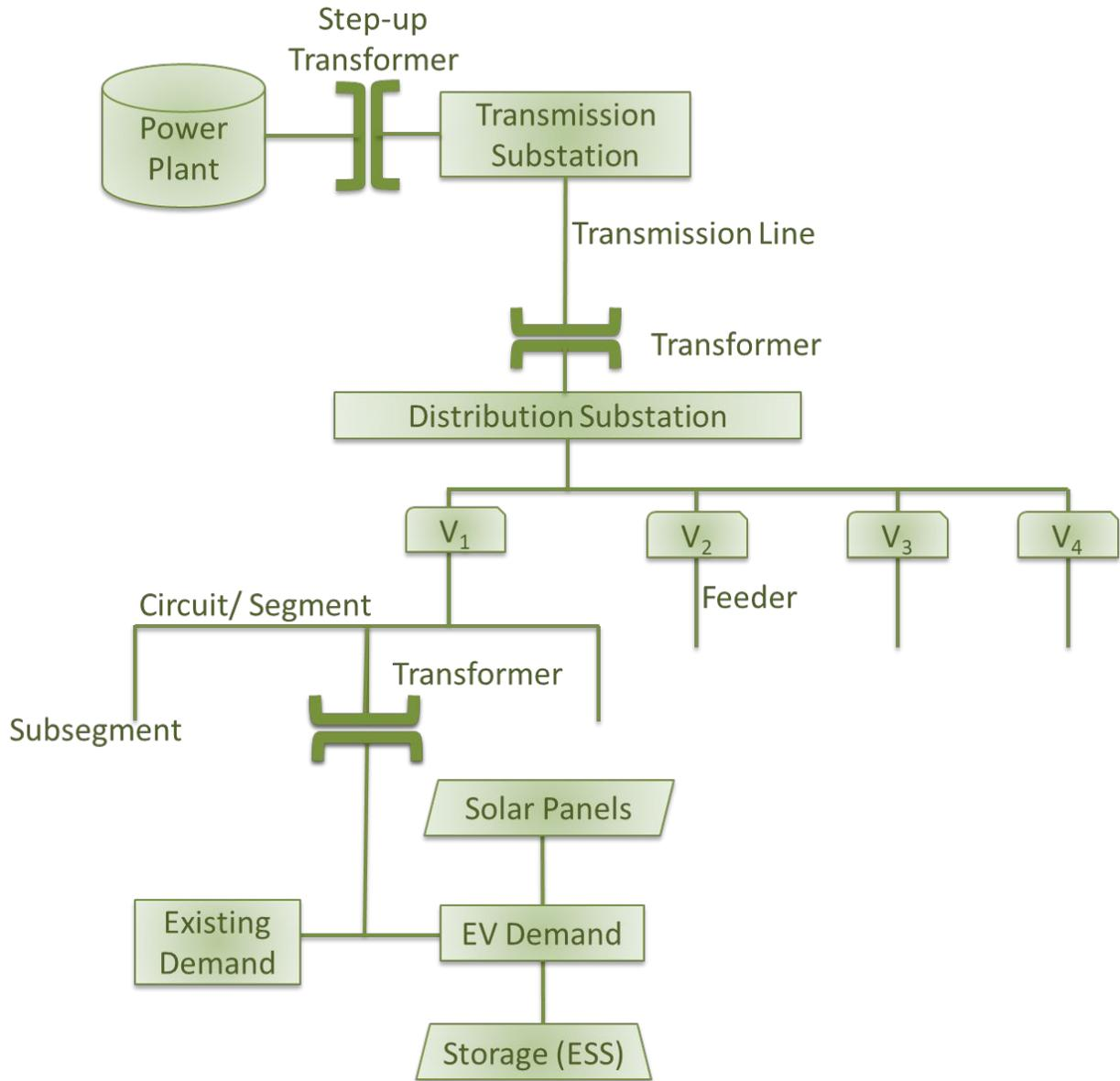
**Figure 1 A schematic description of electric grid network**
