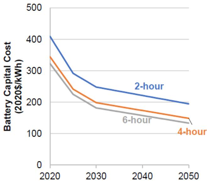
**Figure 3 Projected BESS unit project cost with different storage durations (Cole et al., 2021)**
