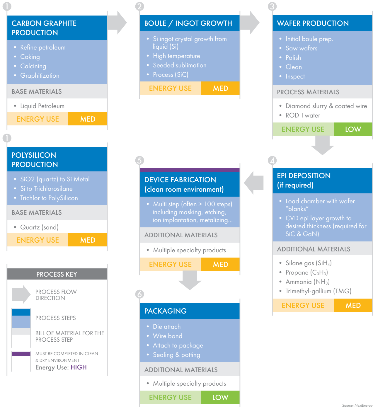
Figure 32: Active Power Device Manufacturing Process
