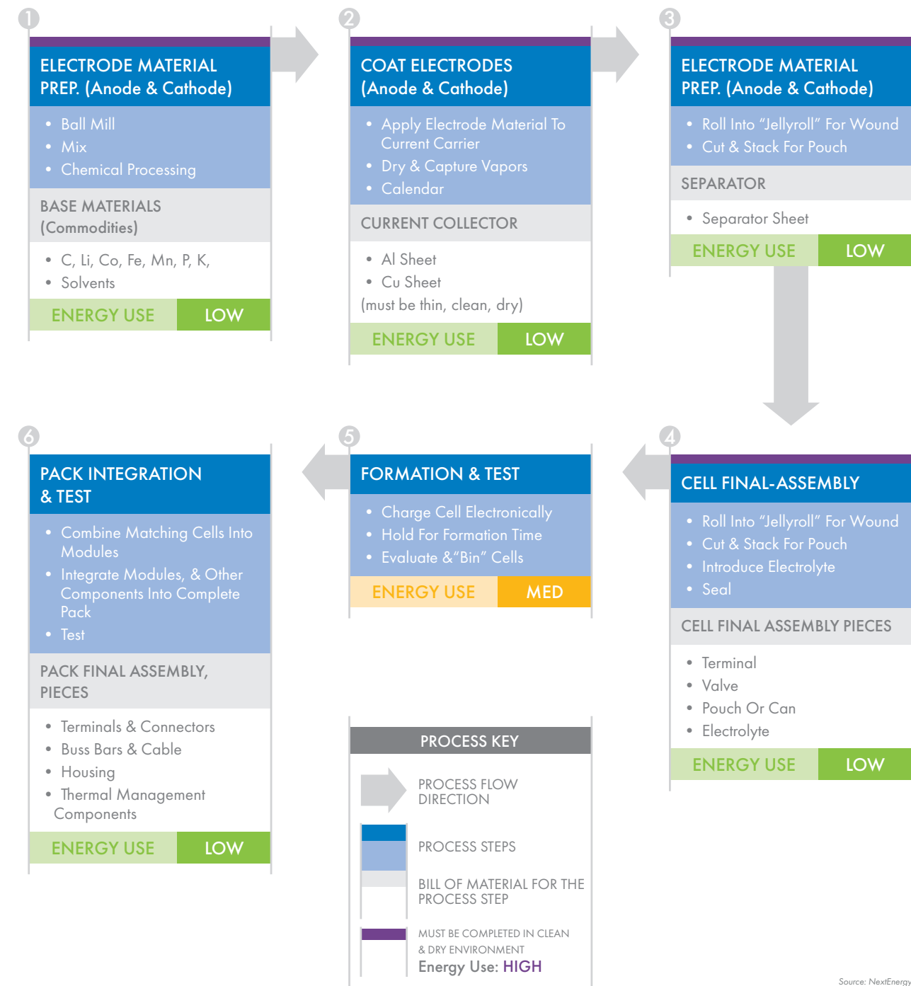
Figure 26: Lithium-Ion Battery Manufacturing Process
