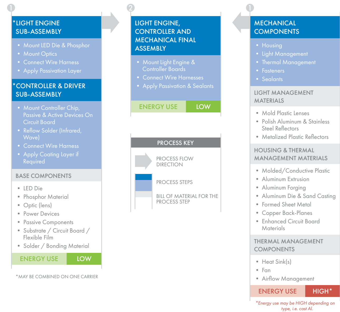
Figure 28: LED Light Engine Manufacturing Process
