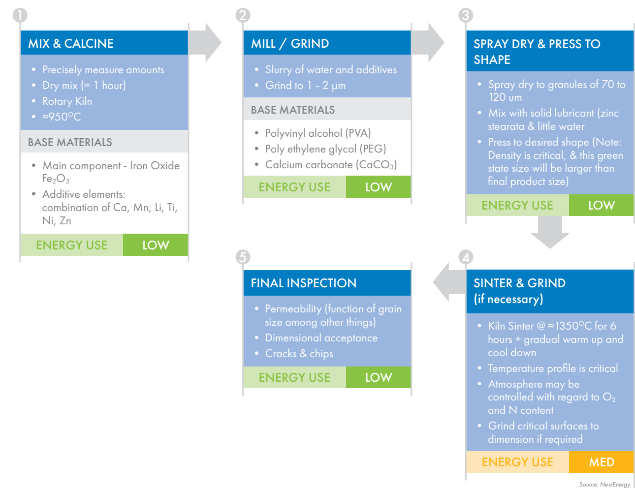
Figure 33: Ferrite Core Manufacturing Process
