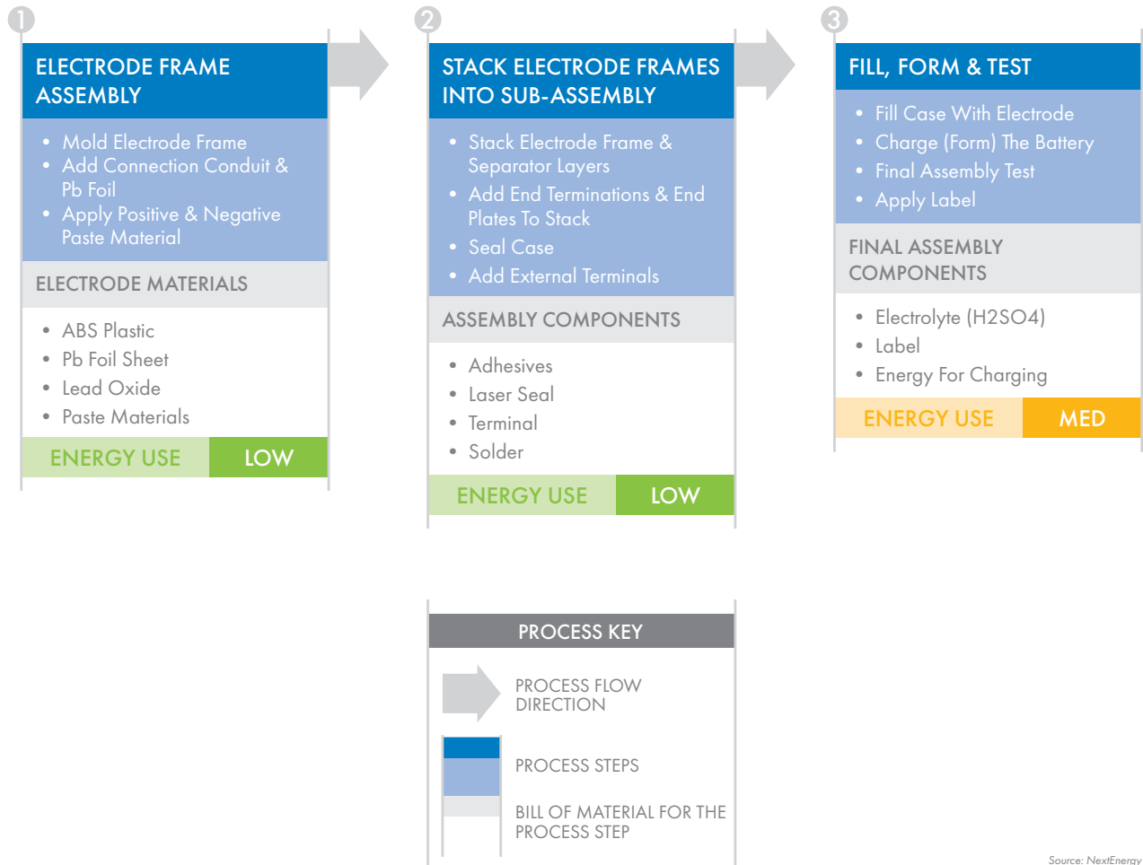
Figure 23: Lead-Acid Battery Manufacturing Process
