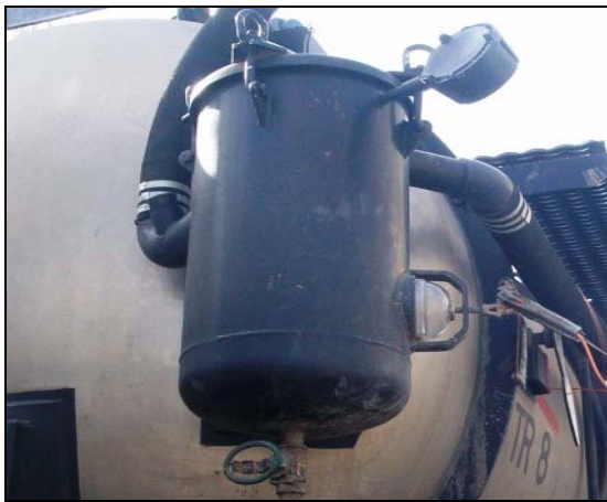
Picture 11 – Muffler & secondary shut off device trap tanks
