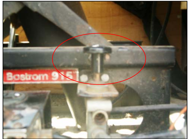
Picture 3 – Emergency switch
