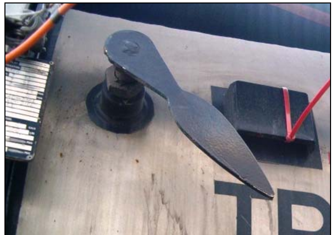
Picture 8 – External float level
