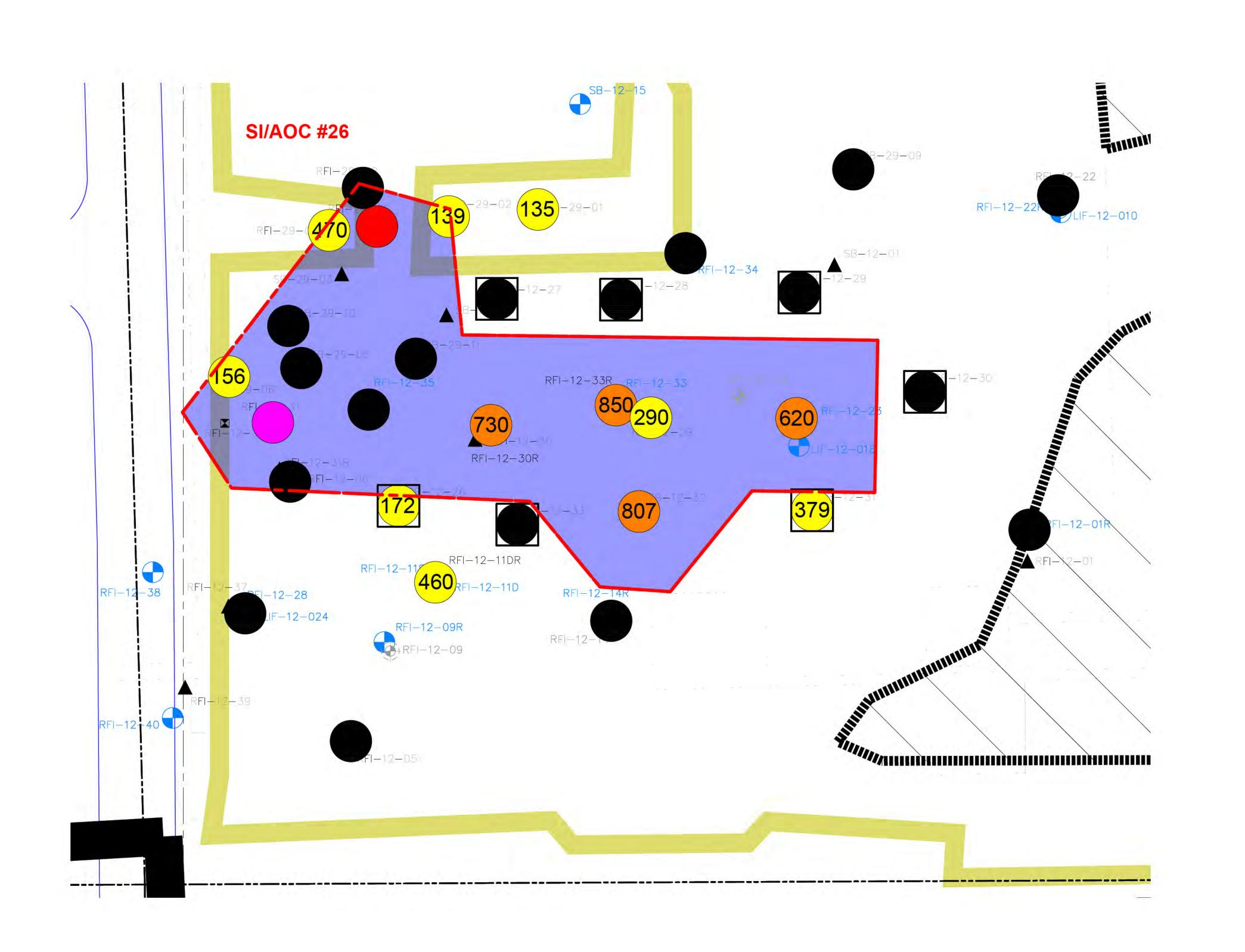
LEGEND: SOIL PILES RESERVED PROPERTIES ---- PROPERTY LINE FORMERLY OWNED RACER PROPERTIES SOIL BORING ABANDONED MONITORING WELL MONITORING WELL (ACTIVE) BORING COMPLETED SINCE 09/22 CONCRETE SLAB PROPOSED AOC EXTENT PROPOSED RESTRICTIVE COVENANT AND AOC EXTENT LEAD >10,000 mg/kg LEAD >5,000 mg/kg, <10,000 mg/kg LEAD >900 mg/kg, <5,000 mg/kg LEAD >600 mg/kg, <900 mg/kg LEAD >100 mg/kg, <600 mg/kg LEAD <100 mg/kg
