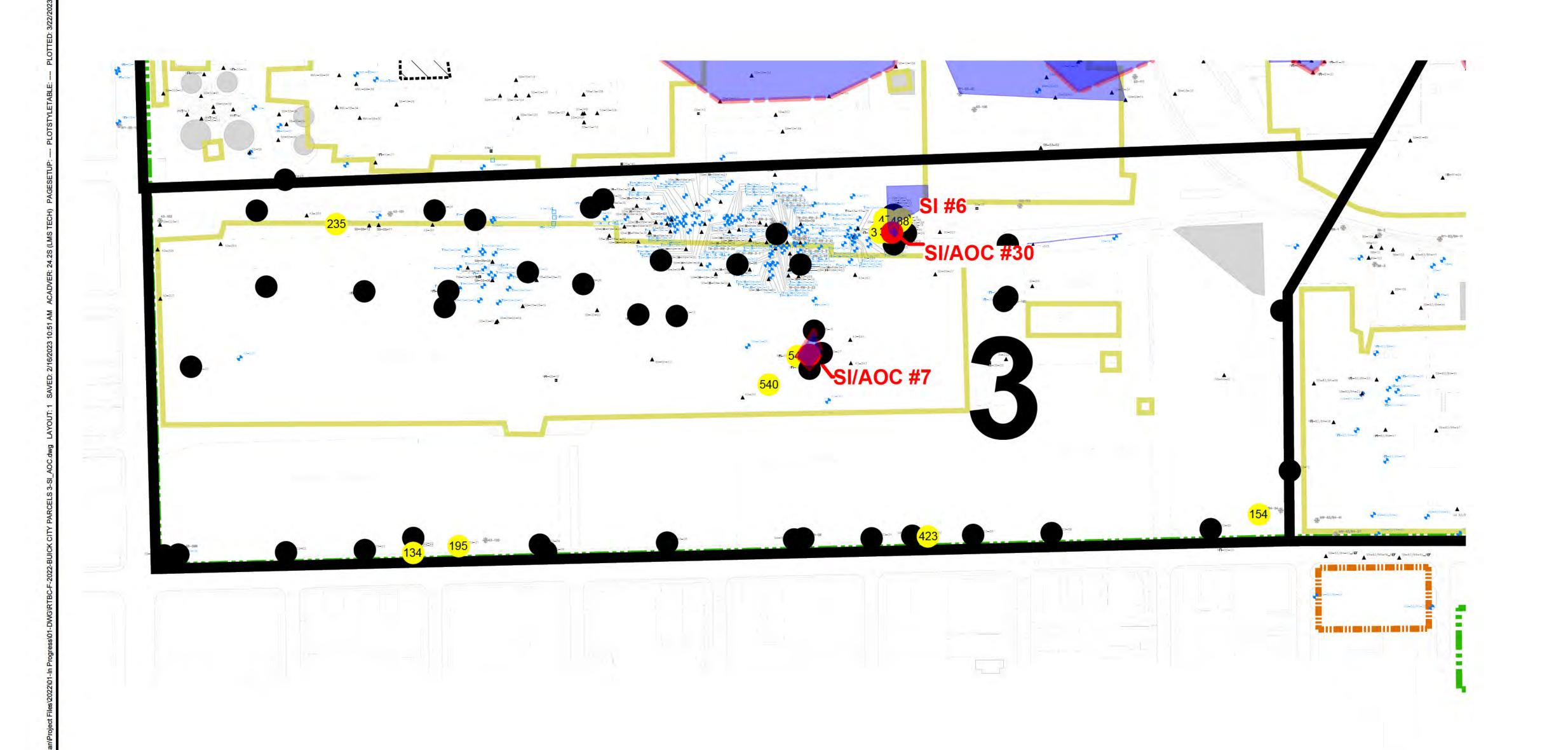
LEGEND: SOIL PILES RESERVED PROPERTIES PROPERTY LINE FORMERLY OWNED RACER PROPERTIES SOIL BORING ABANDONED MONITORING WELL MONITORING WELL (ACTIVE) BORING COMPLETED SINCE 09/22 CONCRETE SLAB PROPOSED AOC EXTENT PROPOSED RESTRICTIVE COVENANT AND AOC EXTENT LEAD >10,000 mg/kg LEAD >5,000 mg/kg, <10,000 mg/kg LEAD >900 mg/kg, <5,000 mg/kg LEAD >600 mg/kg, <900 mg/kg LEAD >100 mg/kg, <600 mg/kg LEAD <100 mg/kg
