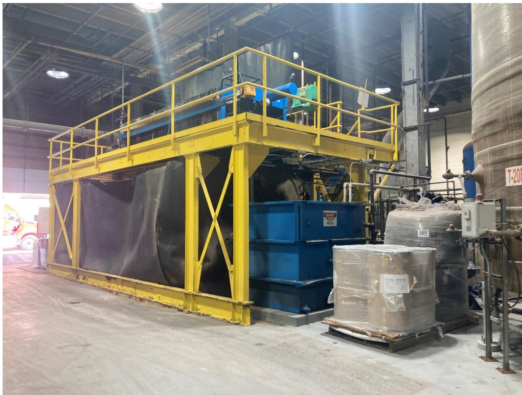
Figure 7. Hazardous Waste Filter Press
