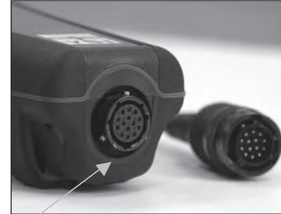
Figure 4, Note the keyed connector.
