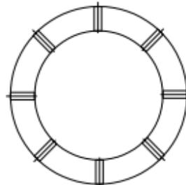
**Figure 2 - MC VI EP2-W Sump Perforation Detail**
