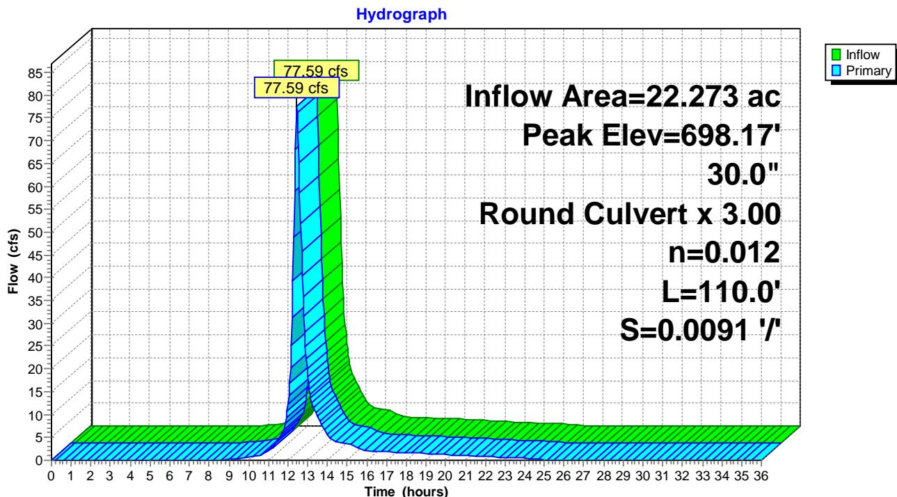
**South Sedimentation Basin (SSB) HYDROCAD OUTPUT – 25-yr, 24-hr**
