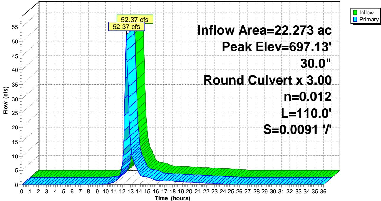
**North Sedimentation Basin (NSB) HYDROCAD OUTPUT – 100-yr, 24-hr**
