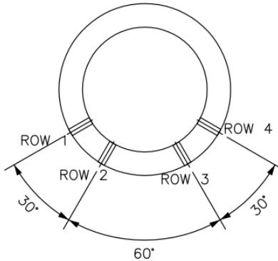
**Figure 2 - Pipe Perforation Detail for MC VI-E, G1 – G3**
