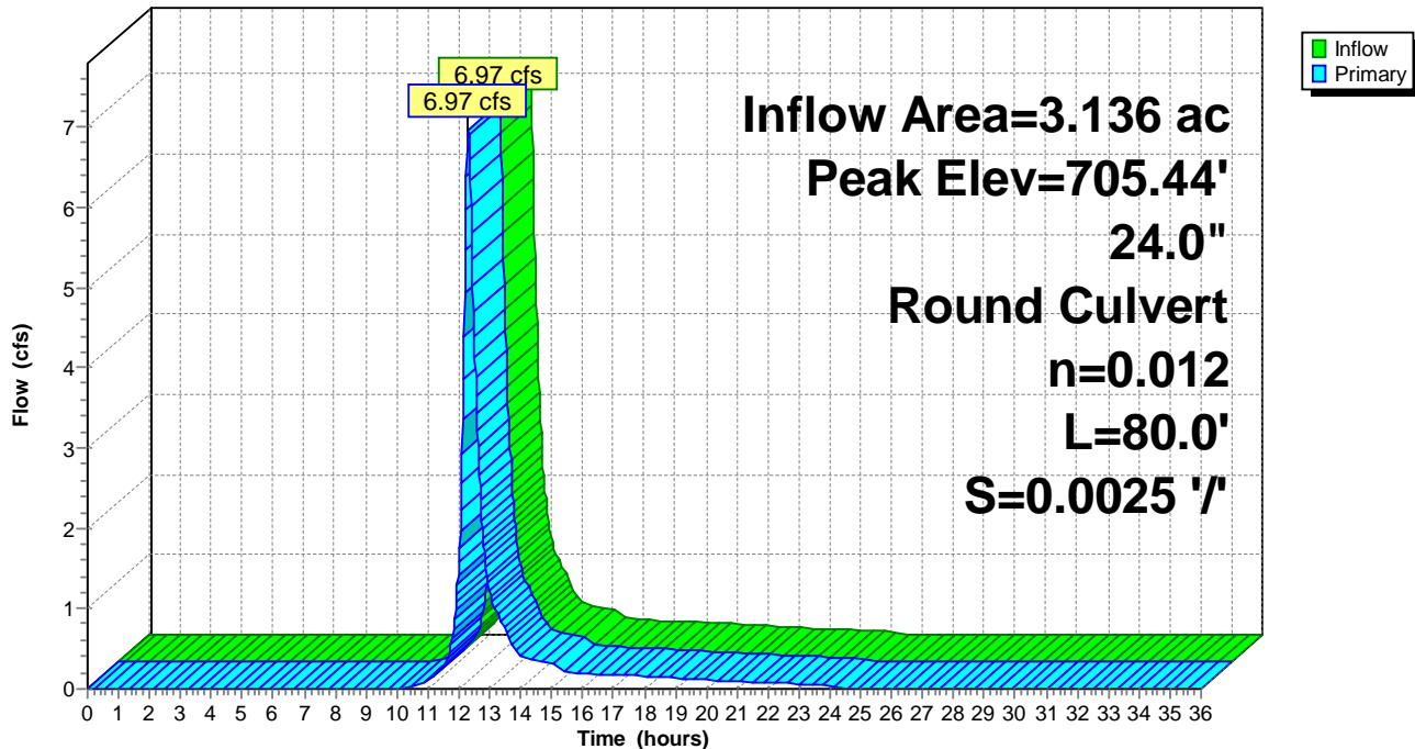
**South Sedimentation Basin (SSB) HYDROCAD OUTPUT – 100-yr, 24-hr**
