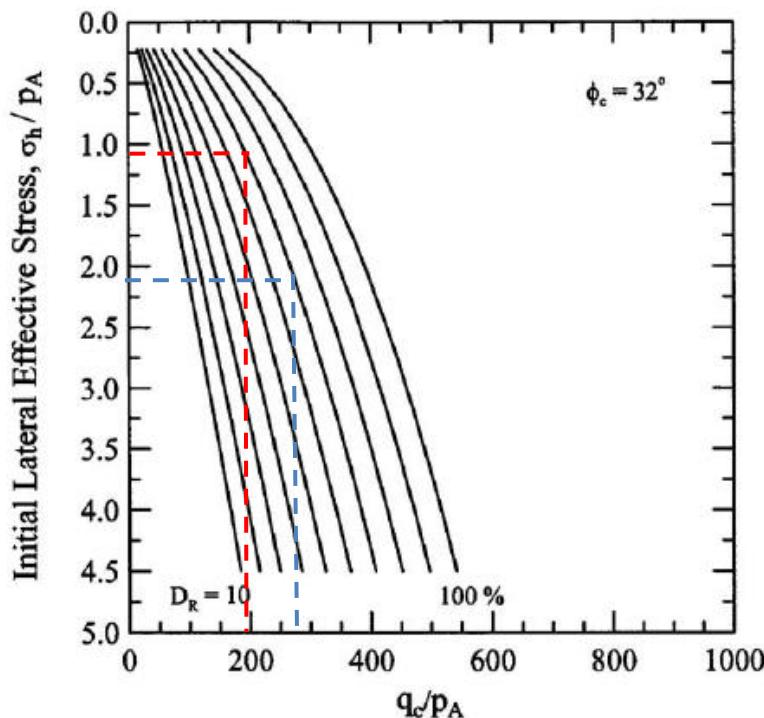
**Figure 1.** Correlation between Stress, Relative Density and CPT value for  $\phi = 32^\circ$
