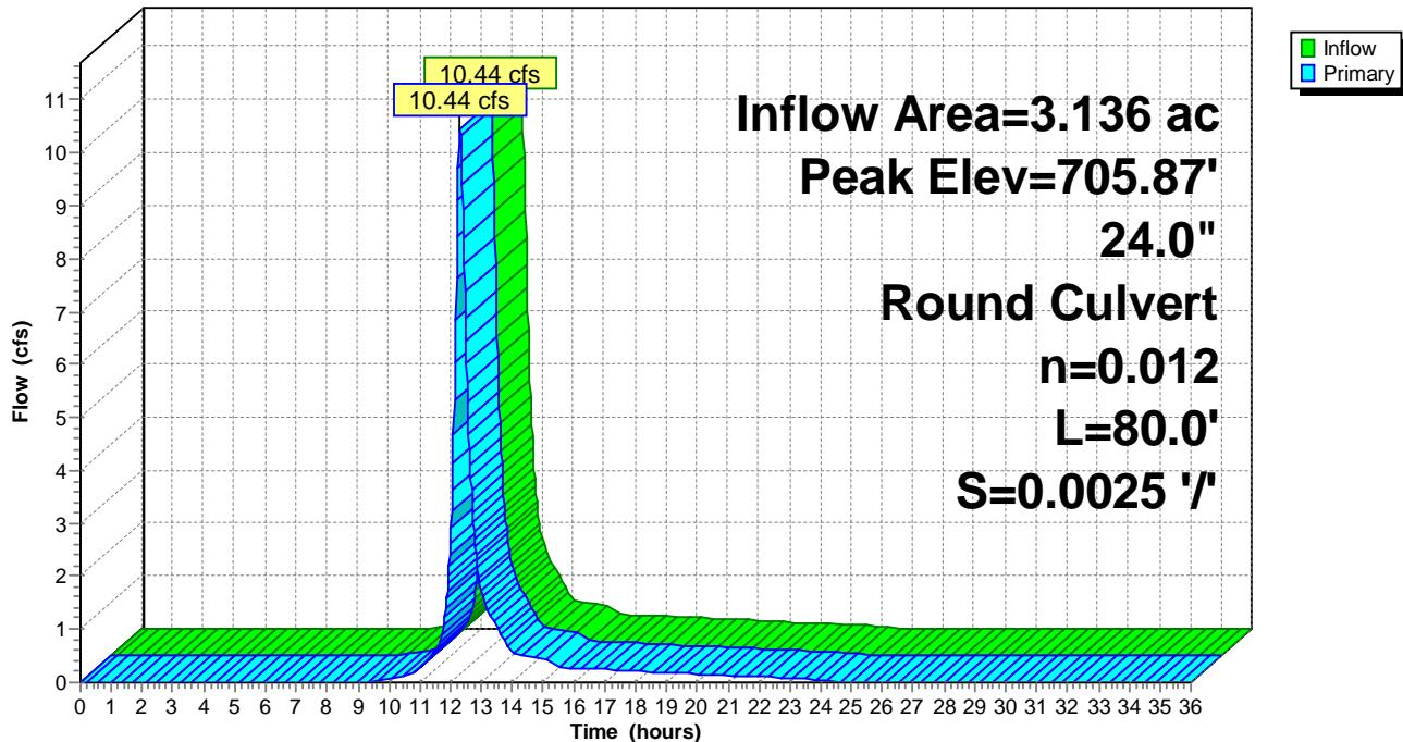
**South Sedimentation Basin (SSB) SWMM OUTPUT – 25-yr, 24-hr**
