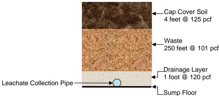
**Figure 3.** Cross Section of Typical Profile of Leachate Pipe for Static Loading Analysis
