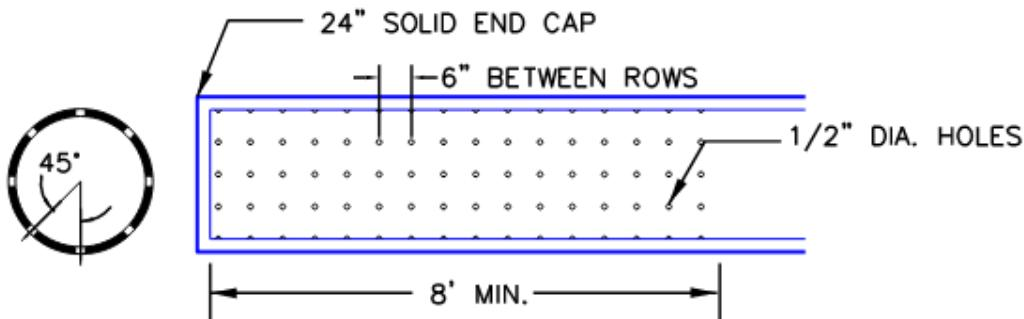
**Figure 1 - Pipe Perforation Detail for MC VI G4 – G7**
