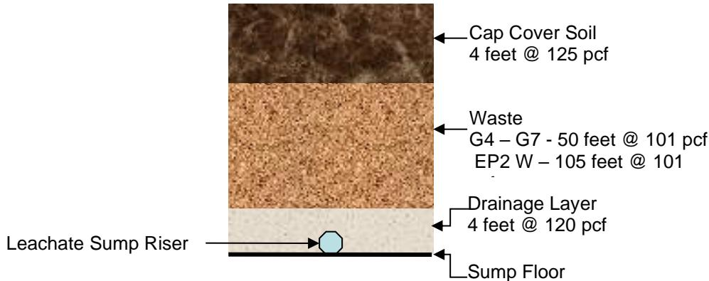
**Figure 3.** Cross Section of Typical Profile of Leachate Pipe for Static Loading Analysis
