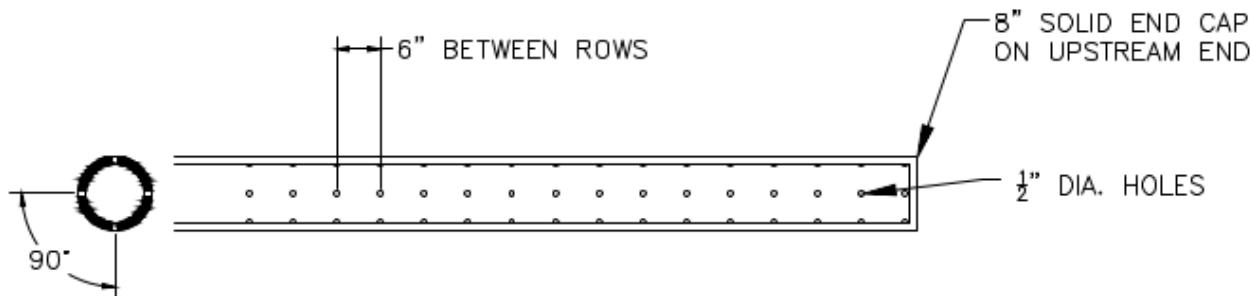
**Figure 1 - Pipe Perforation Detail for MC VI-G4 through G7**
