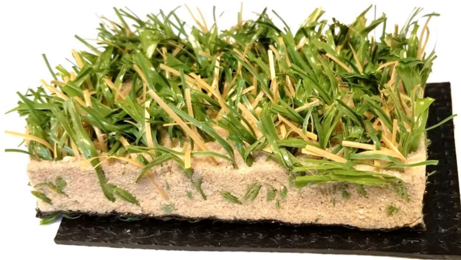
Figure 2 - View of engineered artificial turf with sand infill and textured geomembrane
