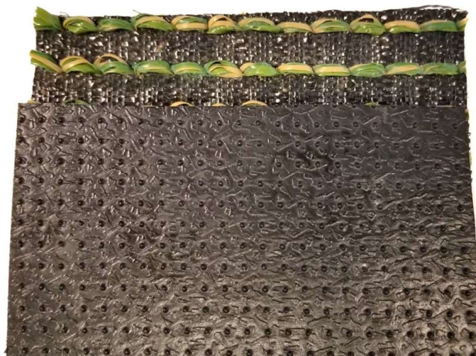
Figure 3 - Underside view of engineered artificial turf and textured geomembrane
