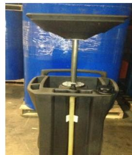
Non-pressurized mobile oil drain pan
