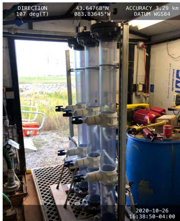
Photo 2: Experimental columns prior to media loading
