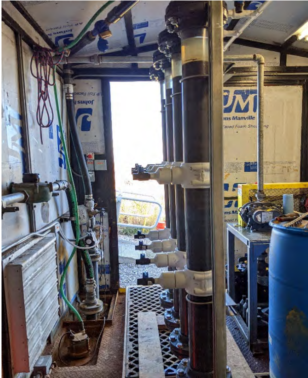
Photo 5: Experimental columns after media loading
