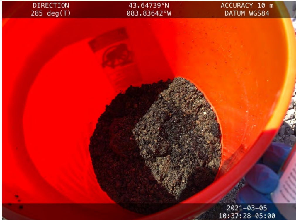
Photo 8: Off-site sand and ZVI mixture after conclusion of experiment
