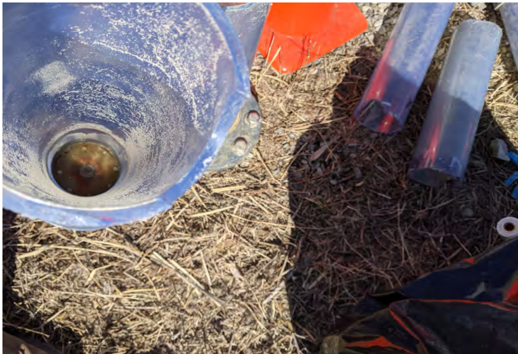
Photo 10: Rust colored build-up on influent screen of an experimental column
