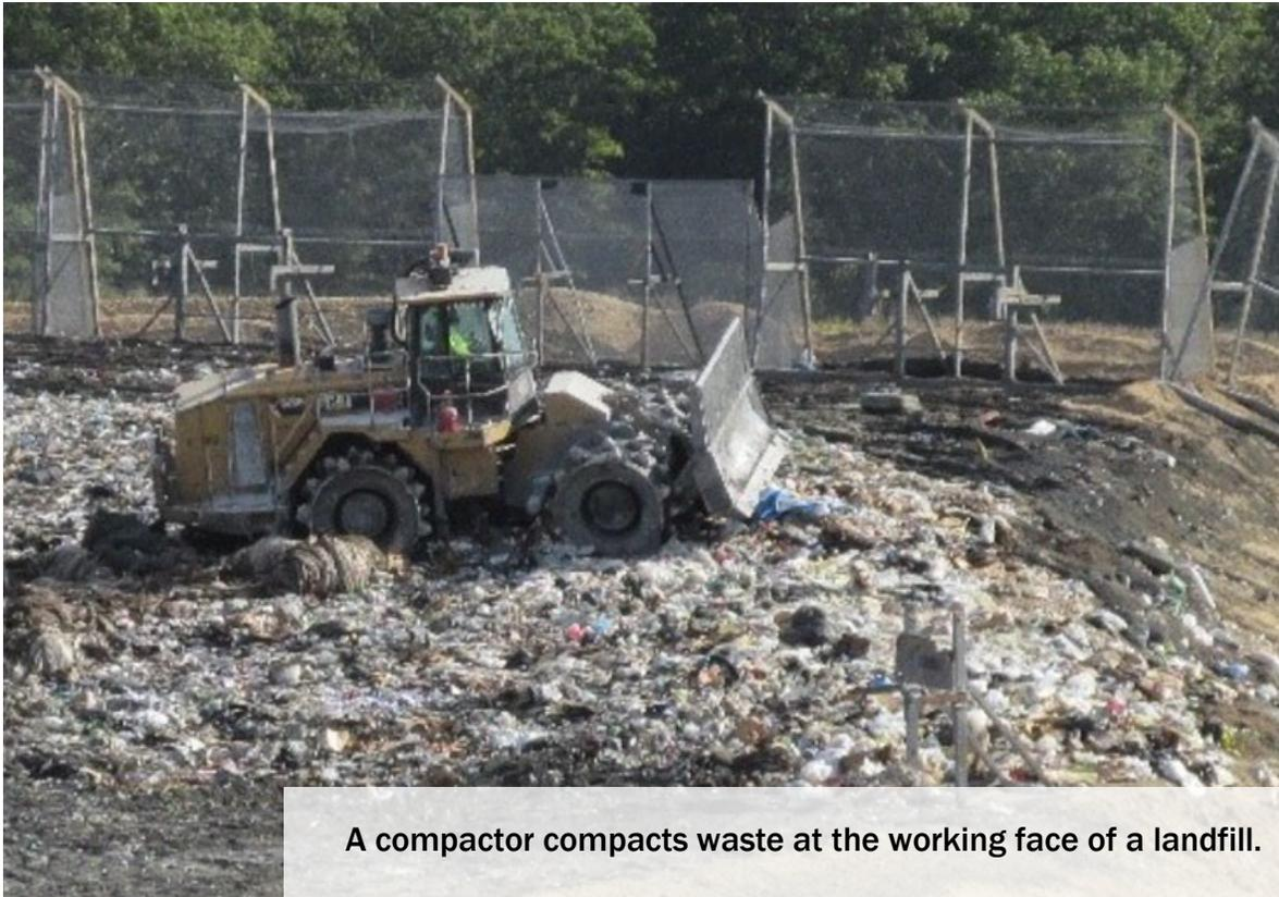
A compactor compacts waste at the working face of a landfill.
