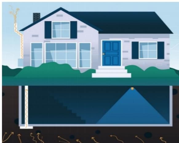
*Radon Mitigation System: House Venting Radon Gas*
