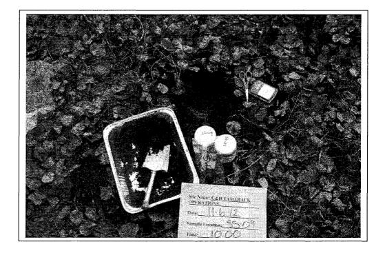
DESCRIPTION: Close-up view of SS-09 sample. Sample was collected at the same location as the XRF-95 screening.
