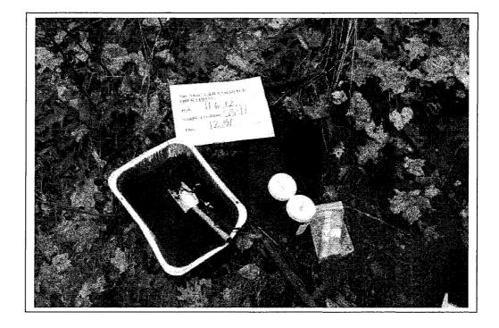
DESCRIPTION: Close-up view of SS-11 sample. Sample was collected at the same location as the XRF-122 screening.
