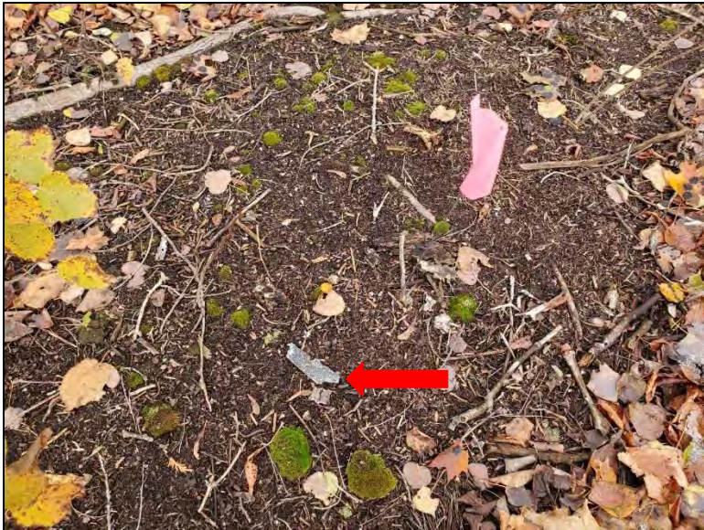
Photo 3: View of damaged ACBM roofing (red arrow) on the ground surface that was removed.
