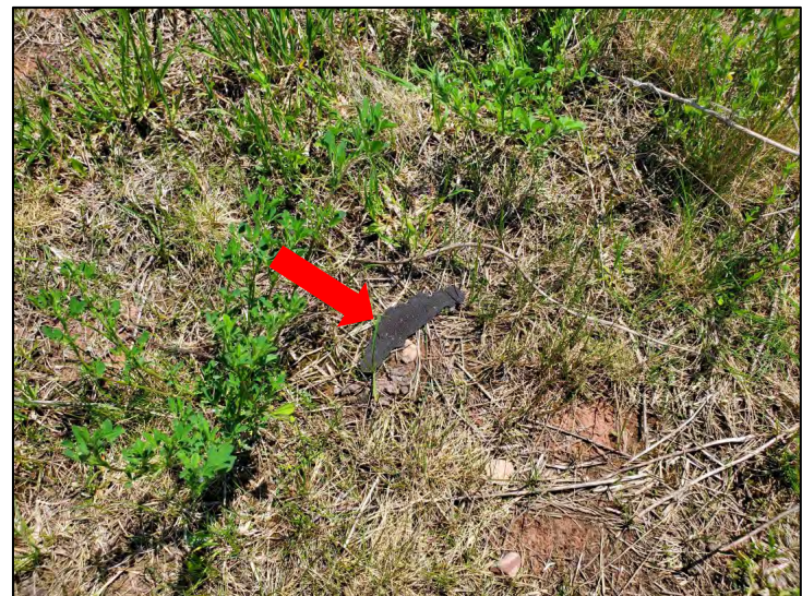
Photo 4: View of a flake of suspect ACBM tar with fibers (red arrow), resting on the cap surface of the Coal Dock Burn Area.
