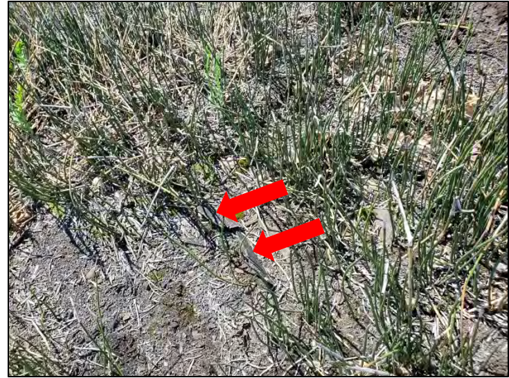
Photo 2: View of ACBM roofing material pieces (red arrows), located on the uncapped area of the Coal Dock Burn Area.
