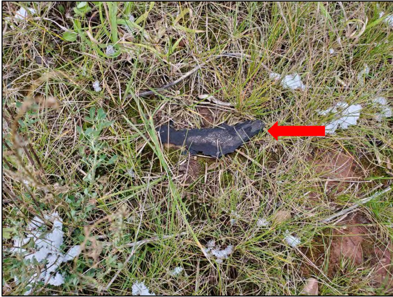
Photo 1: View of tar with fibers SACM (red arrow) scattered on the ground which was removed adjacent to the concrete bulkhead.
