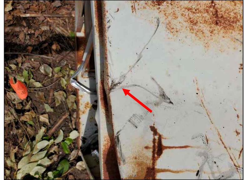
Photo 2: Close up of visible mercury bead on equipment (red arrow). Photo taken on July 17, 2019.
