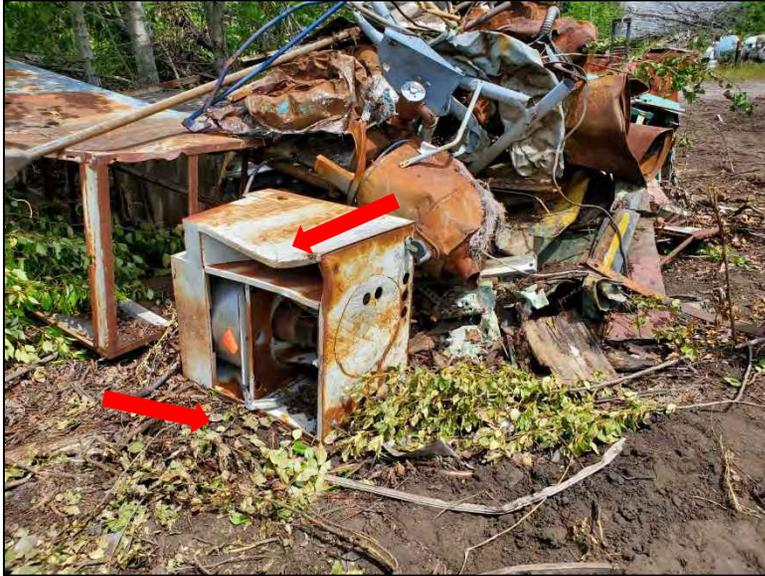
Photo 1: View looking east at scrap metal pile with equipment containing visible mercury beads (red arrows).
