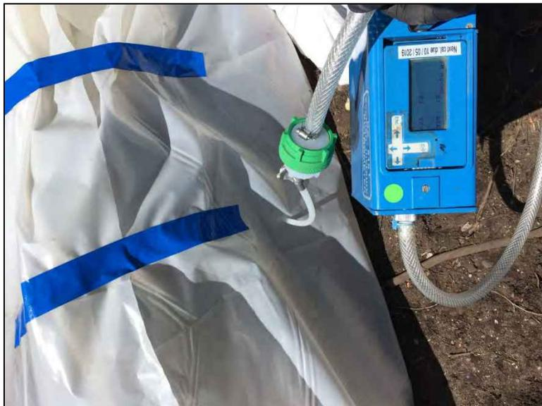
Photo 5: View of scrap encased in plastic to screen for the presence of mercury.
