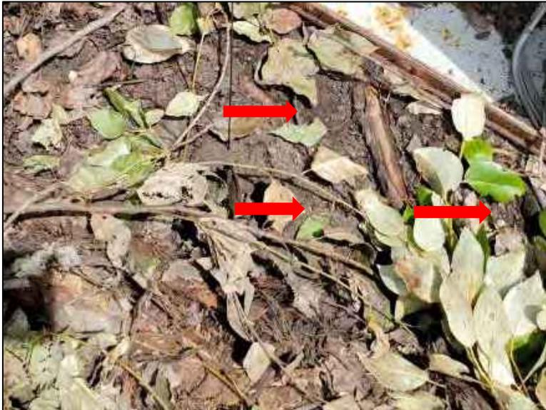
Photo 3: View of small beads of mercury (red arrows) scattered across the ground surface.
