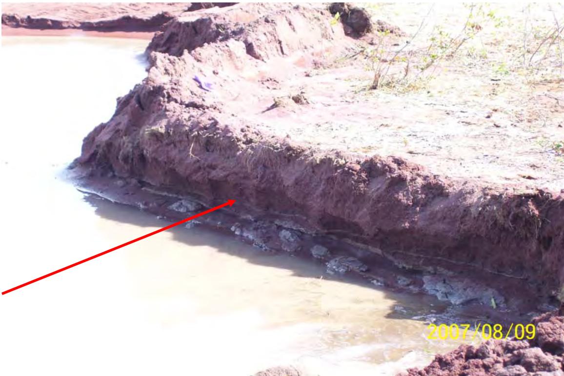
Site: Lake Linden ER Photo Number: 18 Direction: South Subject: Striated, clayey waste material visible below soil surface in Area 1 Date: August 9, 2007 Photographer: NP
