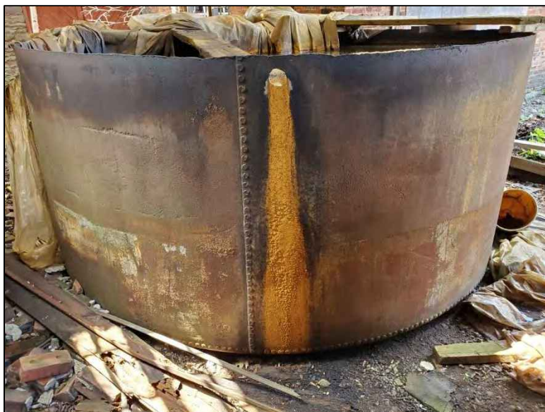
Photo 7: View of a leaking processing vat and stained soil on the ground. Photo taken 7/25/2019.
