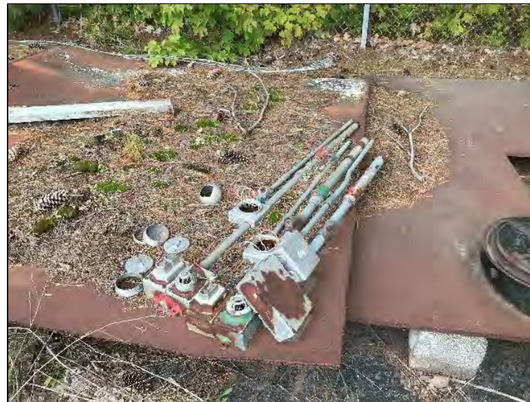
Photo 6: View of potential mercury containing electrical components, identified as observation SHg005. Photo taken 9/27/2018.
