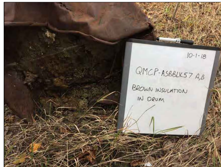
Photo 2: View of brown asbestos insulation stored in an open drum sampled as QMCP-ASBBLK57. Photo taken 10/1/2018.
