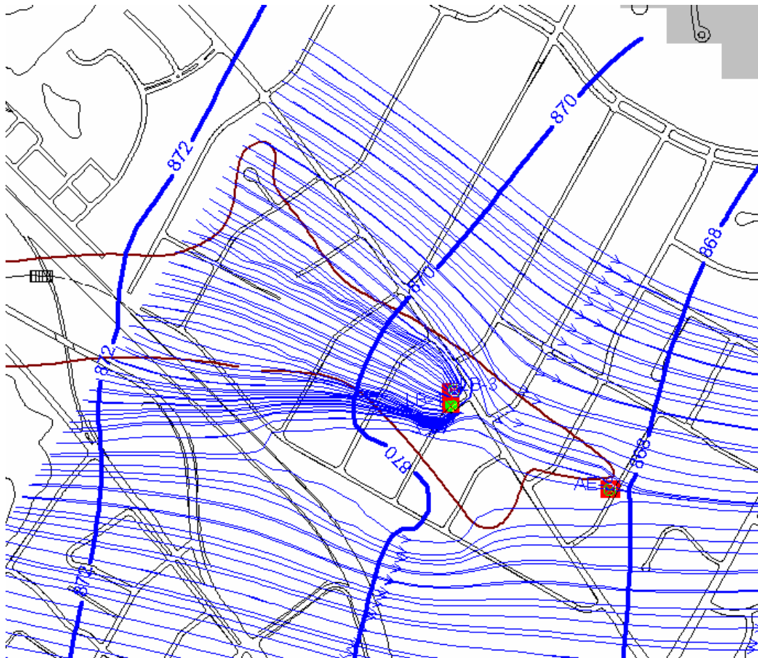
Figure 4 – Steady State Simulation (LB-1 = 45 gpm, LB-3 = 40 gpm, and AE-3 = 10 gpm)
