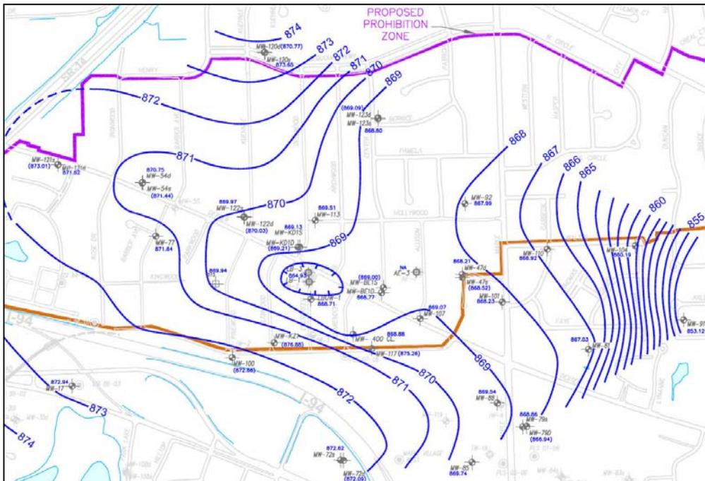
Figure 2 – Potentiometric surface measured May 22, 2009 (Taken from the PLS May22, 2009 map). This map does not use MW-54s, MW-72d, MW-120d, MW-121s, MW-123d, or MW-122d in drawing the potentiometric surface.
