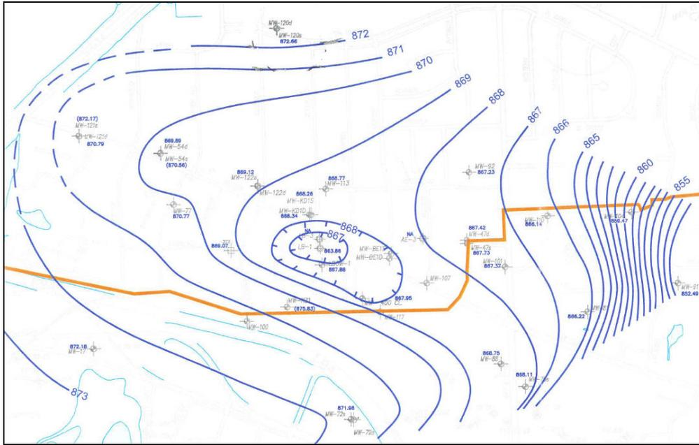
Figure 1 – Potentiometric surface measured January 21, 2009 (taken from the PLS March 2009 report). This map does not use MW-54s, MW-72d, MW-120d, MW-121s, MW-123d, or MW-122d in drawing the potentiometric surface.
