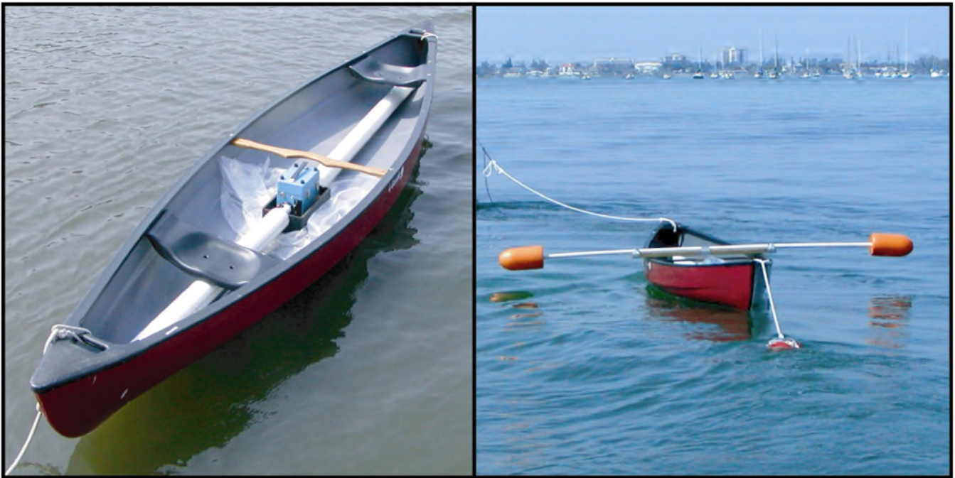
Exhibit 3. Figure from Greenwood (2004) illustrating their way of mounting the EM31 in a non-metallic canoe.
