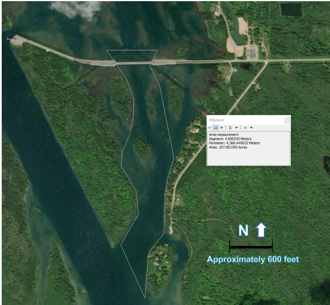
Figure 3. Approximate Little Rapids area restored by new flow regime after bridge construction, as calculated by ArcGIS. Islands within the polygon collectively total about nine acres.
