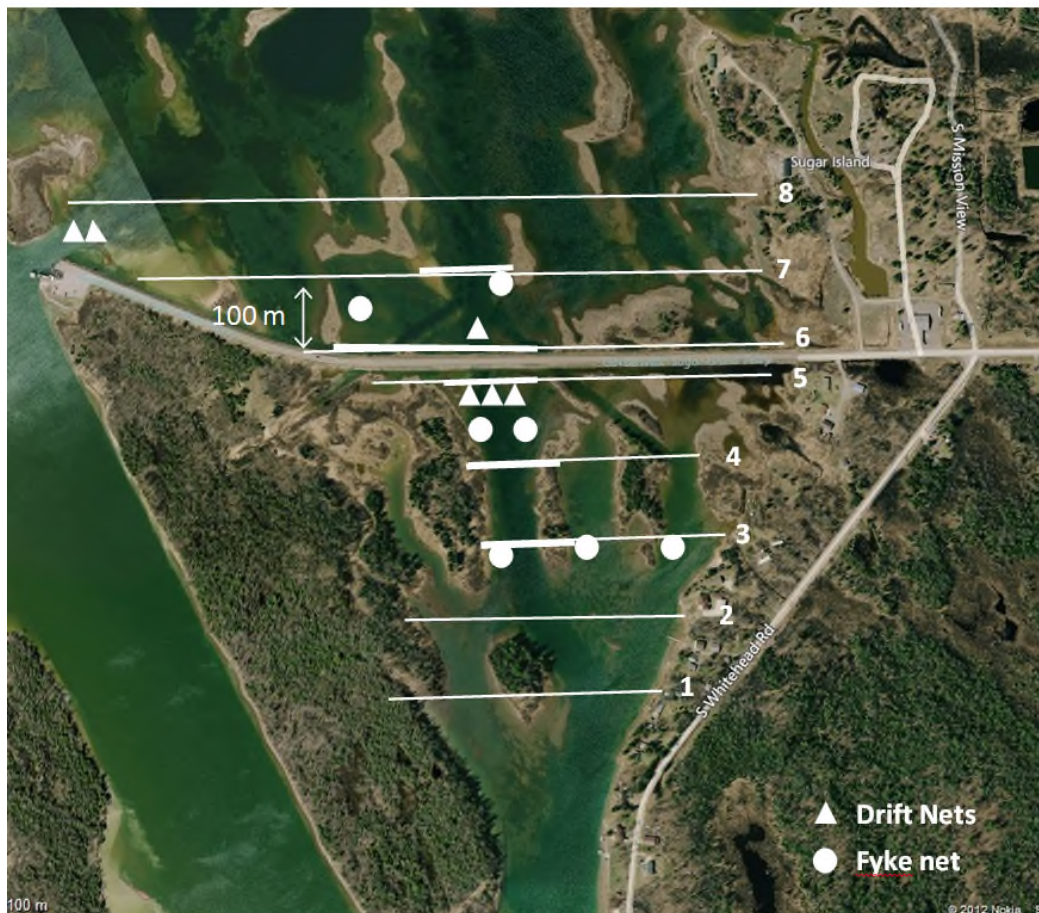
Figure 5. Transects used for monitoring current velocities, fish using drift and fyke nets, total suspended solids (TSS) and macroinvertebrates. The thick lines indicate the locations of velocity measurements. The thin lines indicate macroinvertebrate and TSS sampling, while circles and triangles indicate locations of fish collection gear types. (Image courtesy of A. Moerke, LSSU)
