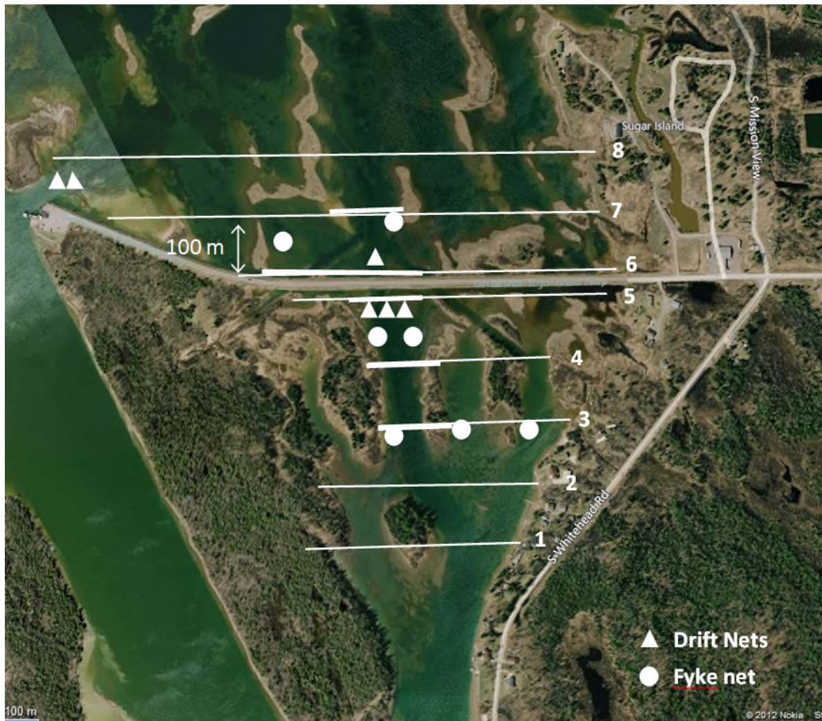
Figure 2. Map of Little Rapids area including location of 100-m transects used for macroinvertebrate and habitat sampling, along with drift net and fyke net locations. Drift nets were limited to areas where flow was sufficient in 2013 and 2014, but they were moved adjacent to the single net on transect 6 after restoration (2017 and 2018) because suitable flow existed. Fyke nets were located in nearshore areas representative of site habitat. The thickened lines on transects 3-7 illustrate locations of current velocity measurements.
