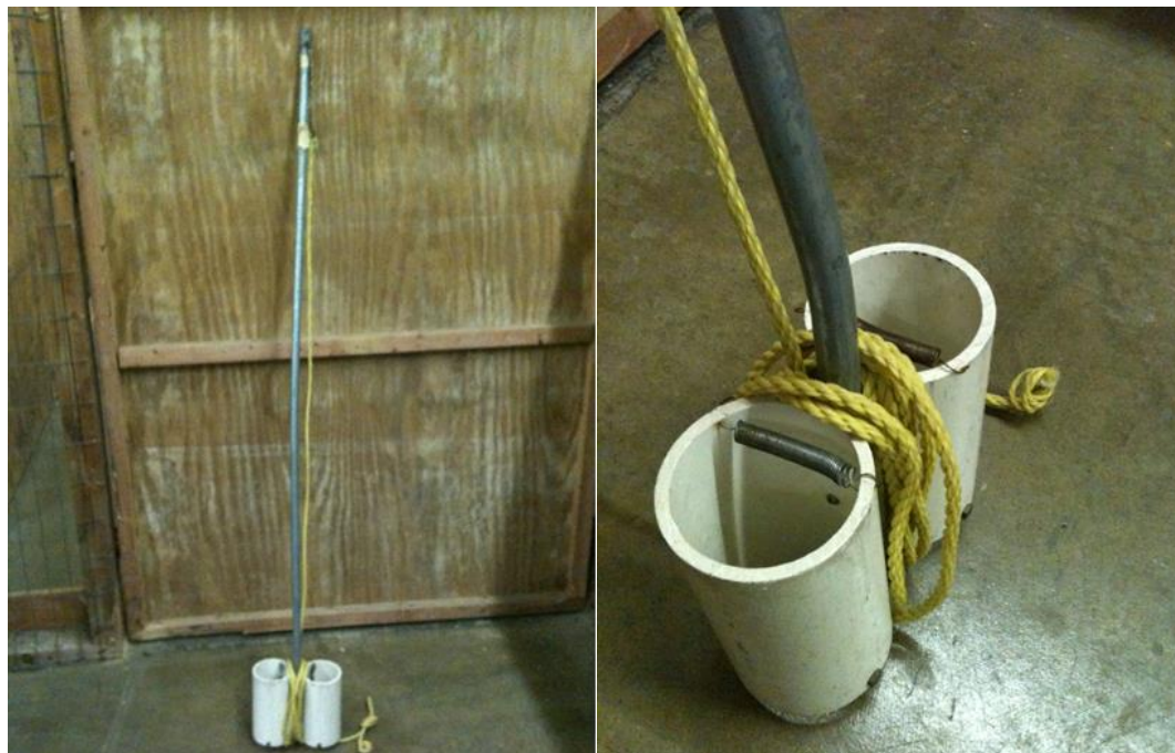
MDEQ-designed “sampling stick”
