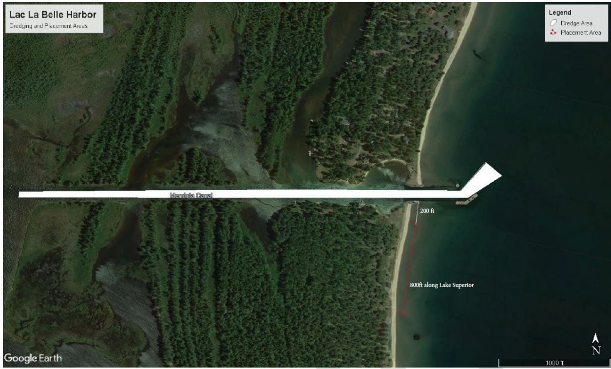
Figure 1. Lac La Belle Harbor dredging and beach nourishment areas.
