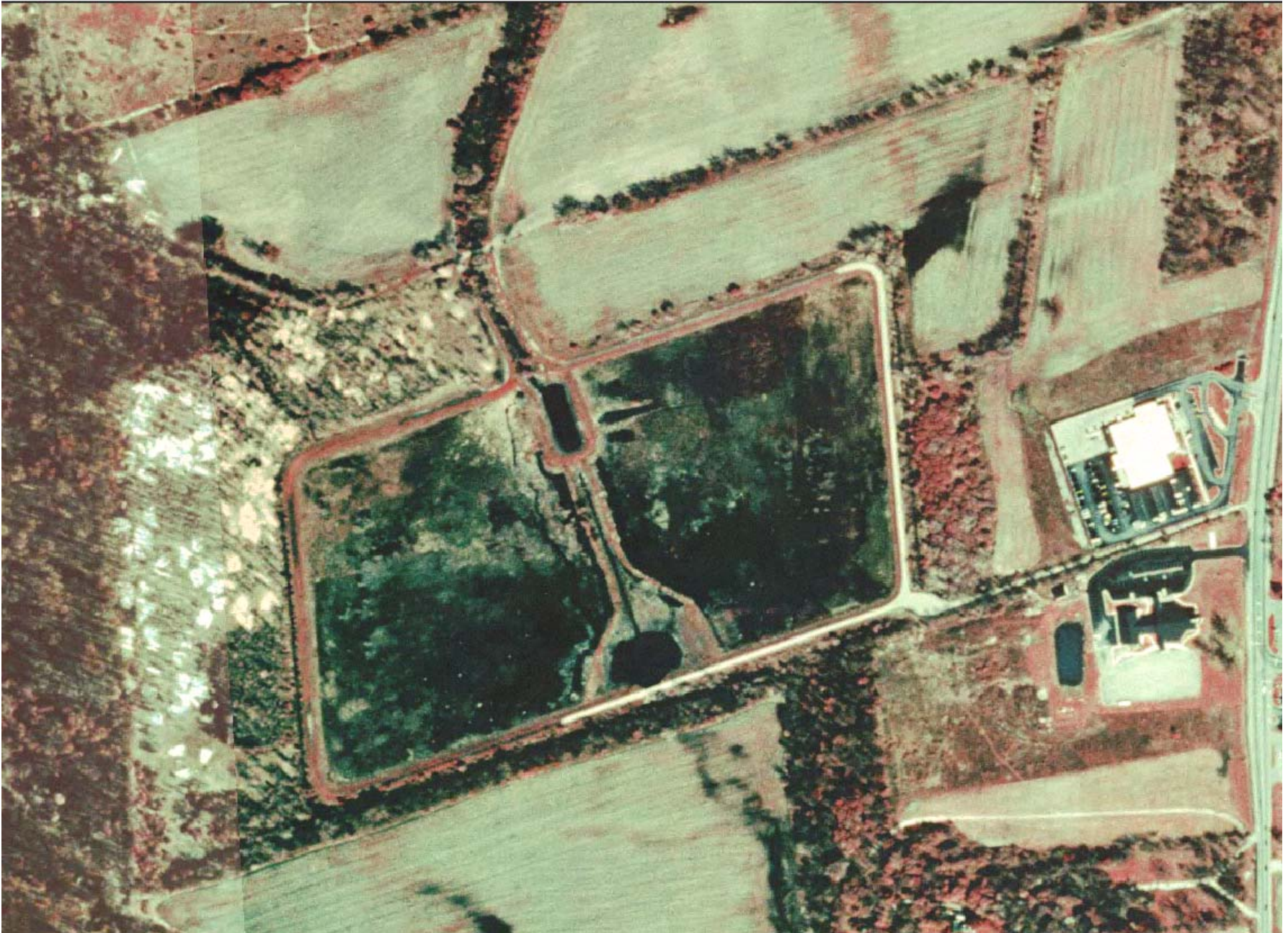
Figure 2. Paint Creek 44 acre detention basin with forebay and micropool (1/2 inch \cong 200 feet).
