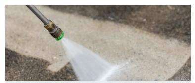
A high-pressure power washing wand substantially reduces the amount of wastewater generated, which means lower transportation and disposal costs compared to washing with a low-pressure hose.
