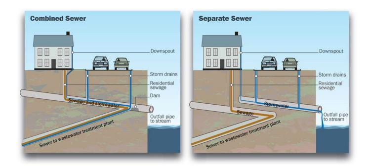
Drains and gutters are typically found outside buildings, in parking lots, or along the streets and usually flow to separated storm sewers or storm drains that lead directly to a stream, lake or other water body. However, some cities, including some very large cities, have combined sewer systems, where storm water is combined with sanitary wastewater and flows to a WWTP. If you cannot verify the sewer destination, then you should not discharge to it.
