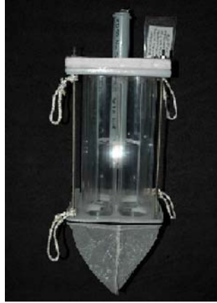
Figure 4. Quatrefoil light trap used for sampling larval fish, micro and macroinvertebrates.
