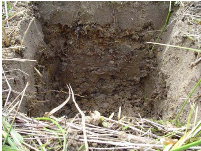
Figure 4. Rhizome and sediment sampling pit: 30 cm X 30 cm X 45 cm. This pit has sand soils underlain by clay soils.
