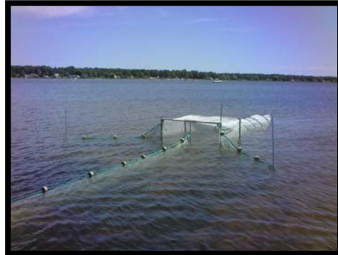
Figure 22. Example of fyke net used to sample adult and juvenile fish. Six nets were set at each paired site.
