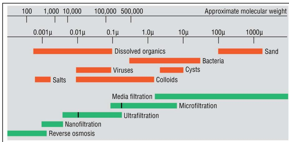
Nanofiltration (NF) membranes typically have pore sizes of 0.001 microns and an MWCO ranging from 1,000 to 100,000 Da. NF membrane systems is used for the removal of selected dissolved constituents from wastewater such as the multivalent metallic ions (hardness), and a fraction of the monovalent species (sodium and chloride).
