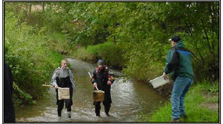
Wayland New Directions Program, Red Run Drain at North Dorr Park: Students sample and identify macroinvertebrates. Numbers and types are recorded to quantify stream condition and water quality.
