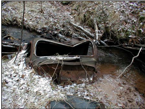
Site #16 - Badger Creek (before). Vehicle was impounding the creek and starting to scour away the stream bank.
