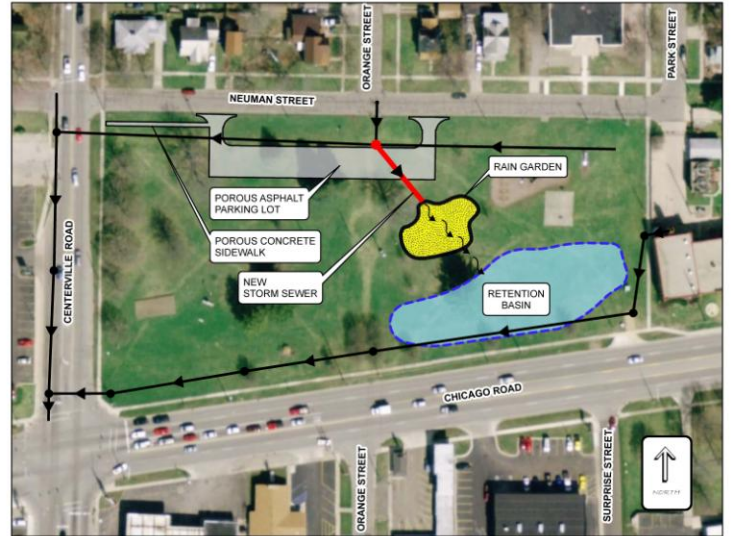
Memorial Park (After): A storm sewer from the residential neighborhood was diverted to the park. A porous sidewalk and parking lot, rain garden, and a retention basin were installed to infiltrate storm water runoff on site.
