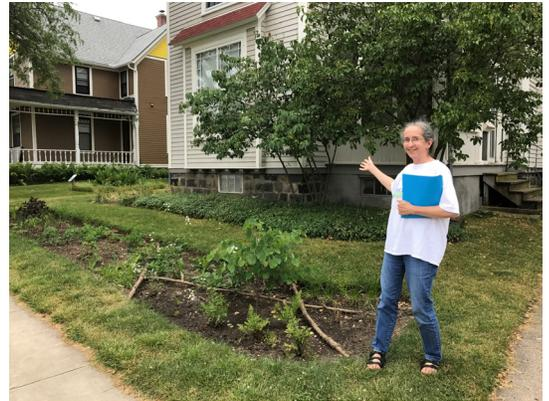
**Pat Martz front yard After:** By taking the Master Rain Gardener class, resident Pat Martz designed a 160 square foot rain garden to capture the roof runoff from two downspouts, capturing water from 800 square feet of roof. The rain garden included Nodding Wild Onion, Liatris, Blue Flag Iris, Wild Geranium, Foam Flower, Culver's Root, Wild Ginger and an Alternate-Leaved Dogwood.
