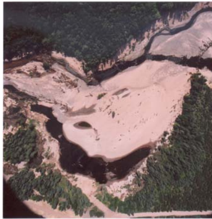
Figure 1. Aerial photographs of sediment deposition in the floodplain 2 months after the dam failed.
