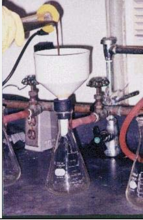
Determination of Mixed Liquor Suspended Solids (MLSS) and Mixed Liquor Volatile Suspended Solids (MLVSS)
