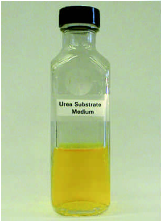
Photo 4. Urea Substrate Medium. After adjusting the pH of the medium to 3–4, the Urea Substrate Medium should be straw-yellow in color.
