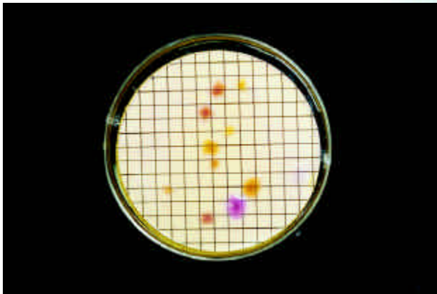
Photo 6. Escherichia coli colonies on an absorbent pad saturated with Urea Substrate Medium. E. coli colonies remain yellow, yellow-green, or yellow-brown when the filter is placed on the Urea Substrate Medium, while nontarget colonies turn pink or purple.
