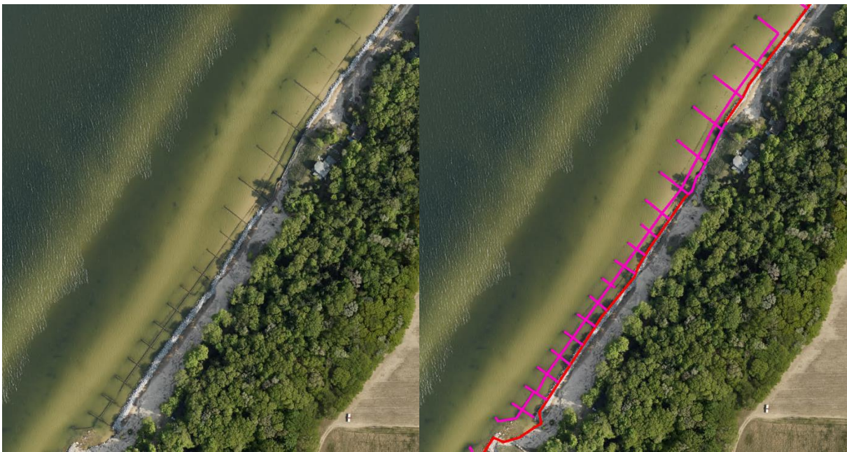
Figure 16. Shoreline hardening visible in 2020 aerial imagery (left) and mapped (right)
