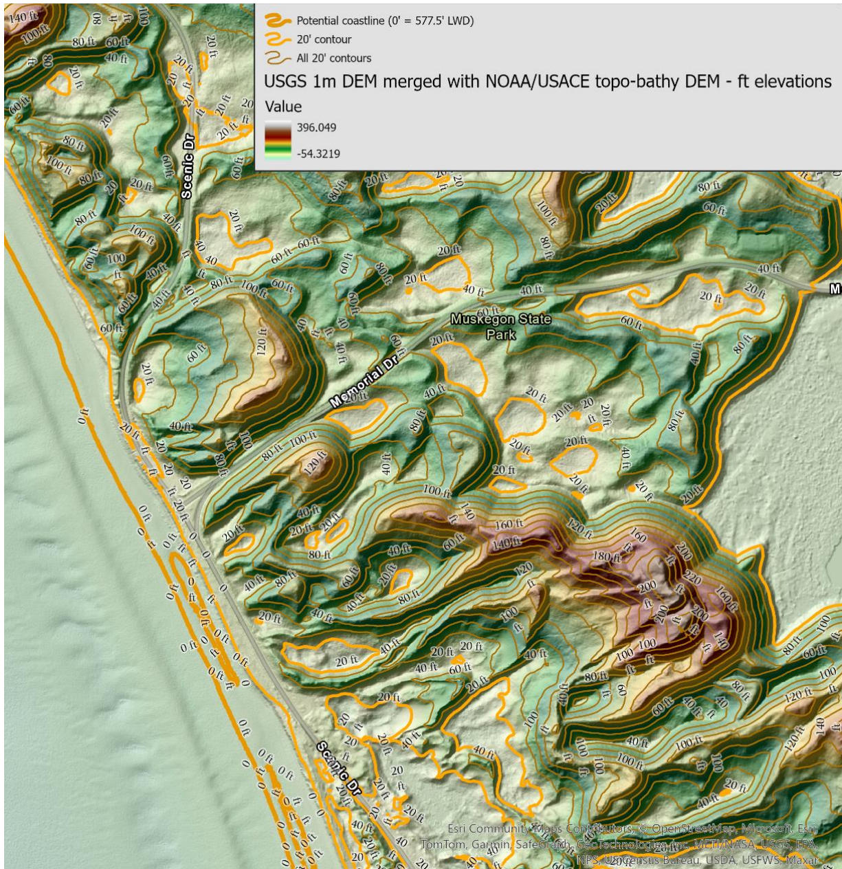
Figure 2: Merged DEM combining the USGS one-meter DEM with the USACE/NOAA coastal topobathy DEM for an area of Muskegon State Park, with example elevations based on a zero-foot contour at the LWD of 577.5 feet.
