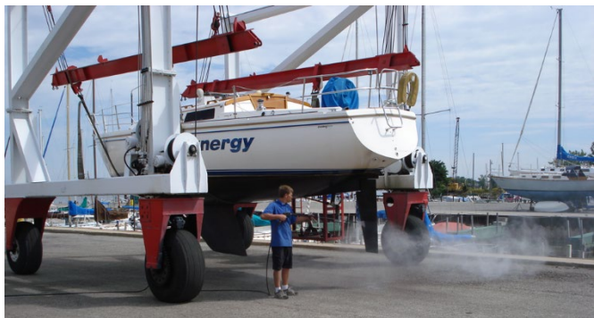
Figure 41 - Wastewater from vehicle washing is not authorized under the storm water permit.
