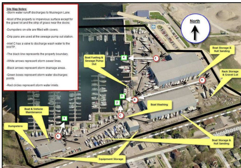
Figure 12 – The SWPPP site map needs to include all items listed under the site map requirements in the permit.
