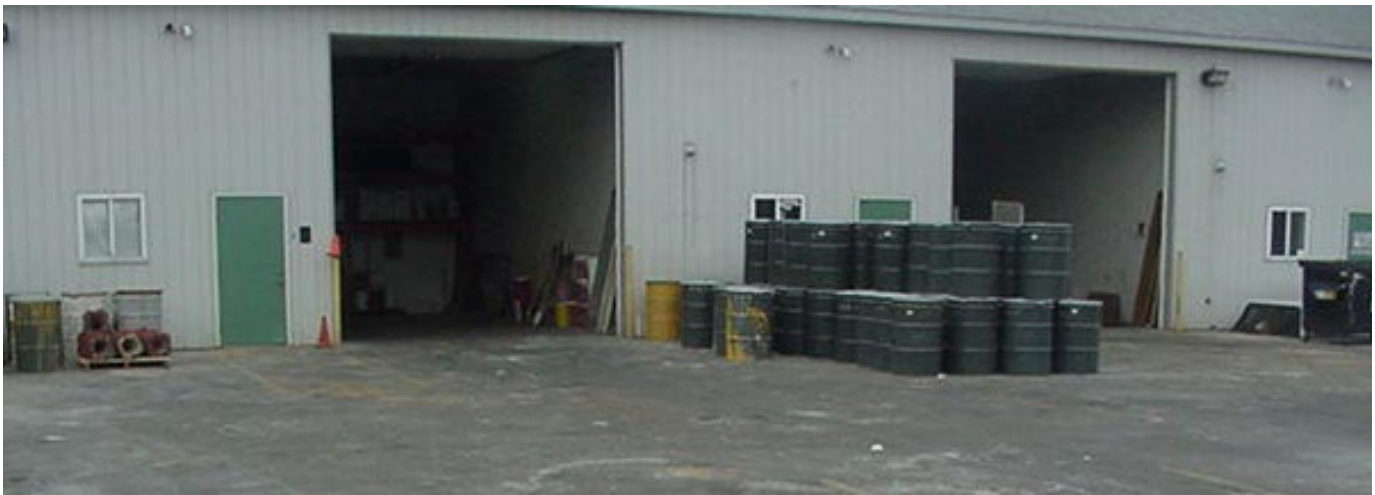
Figure 14 – Facilities need to develop an inventory of their significant materials that could be exposed to storm water.
