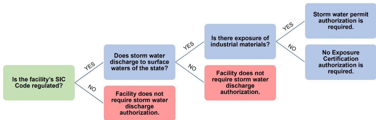
Figure 8 - Flow chart to help determine what type of industrial storm water authorization is required.
