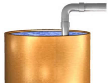
Typical Cross-Connection - Submerged Inlet
