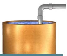
Typical Cross-Connection -Submerged Inlet
