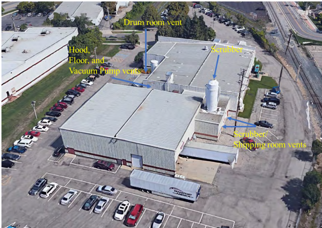
Figure 4 – Vent and Stack Locations at Facility
