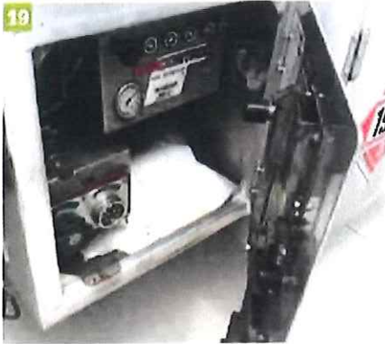
(18) Manual belly valve controls on a four-compartment tanker. (19) Pneumatic belly valve controls on a five-compartment tanker. Note the two black plungers on the door that release the corresponding actuators when the door is opened. The actuators simultaneously lock the trailer brakes and open the top vapor valves. Also note the thermistor/optic plugs in the lower left for static control at the loading rack.
