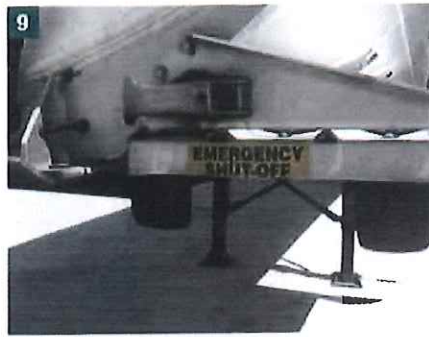
(9). The emergency valve, which closes all the belly valves on the trailer. (Photo by author.)
