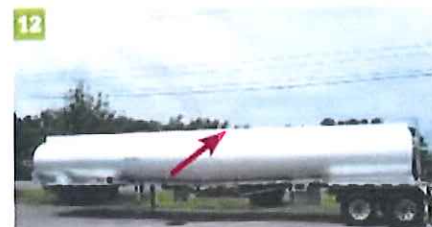
(11) A vent hole between a double bulkhead. (12) A typical MC-406 tanker trailer. Along the top is the eight-inch overturn protection rail (arrow) through which runs the vapor recovery system and the access ladder at right.
