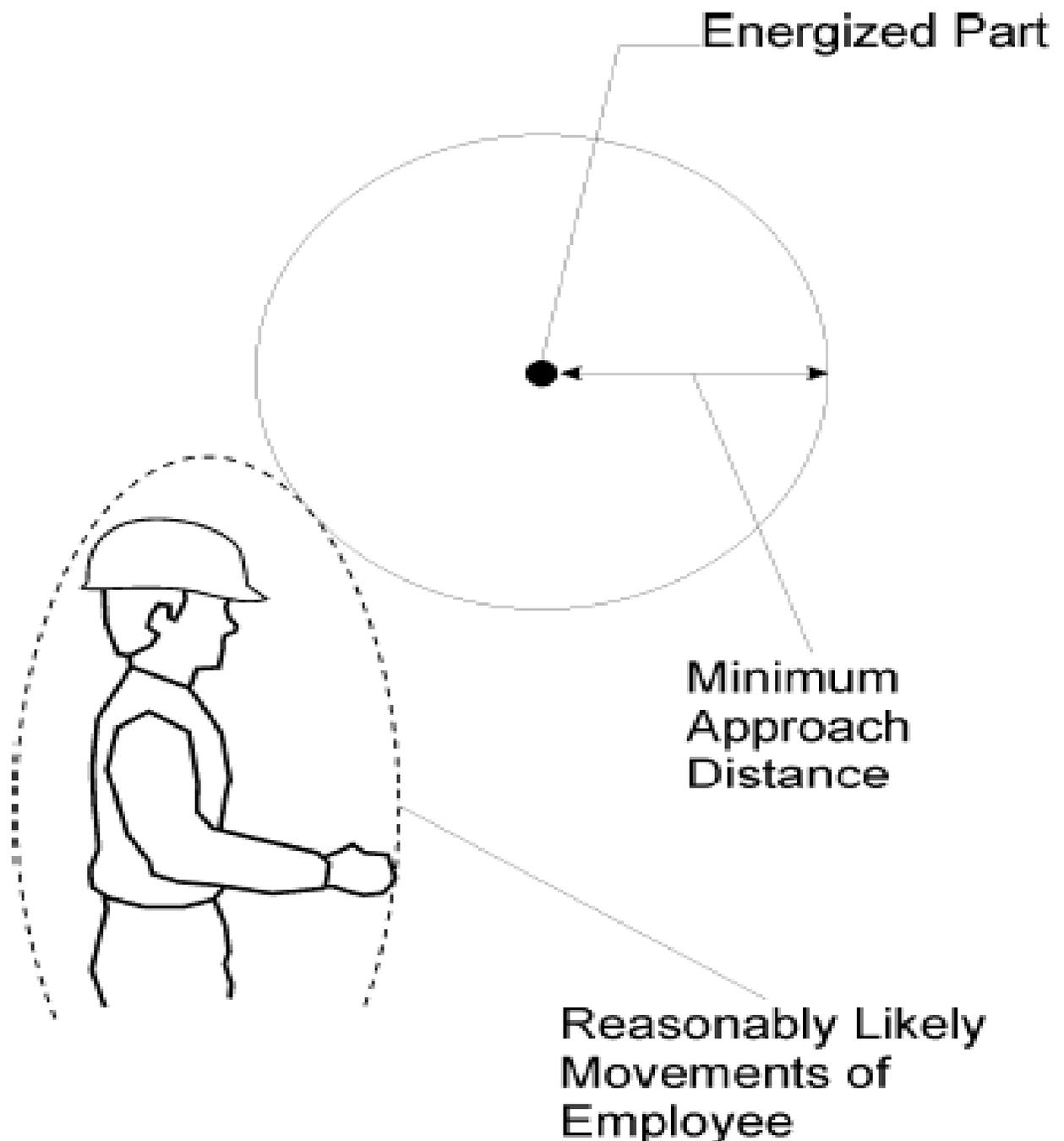
Figure 1 – Maintaining the Minimum Approach Distance
