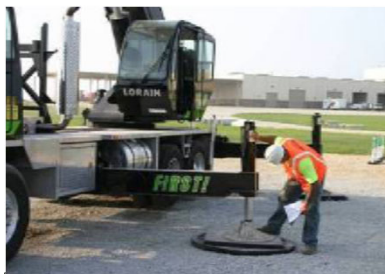
Outrigger or stabilizer pads and floats for excessive wear or cracks.
