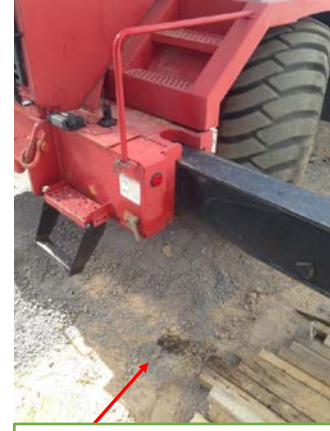
Wet spot indicates possible hydraulic leak.
