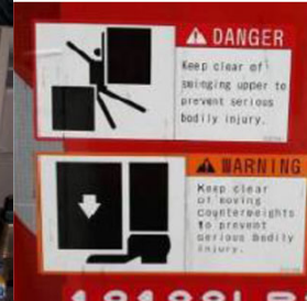
Missing or unreadable warning labels and decals.
