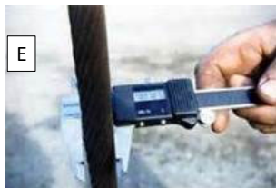
Micrometer checking diameter of wire rope.
