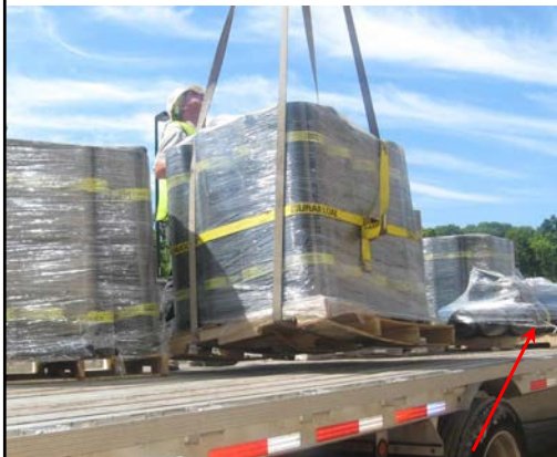
Note the deformation of the pallet.
